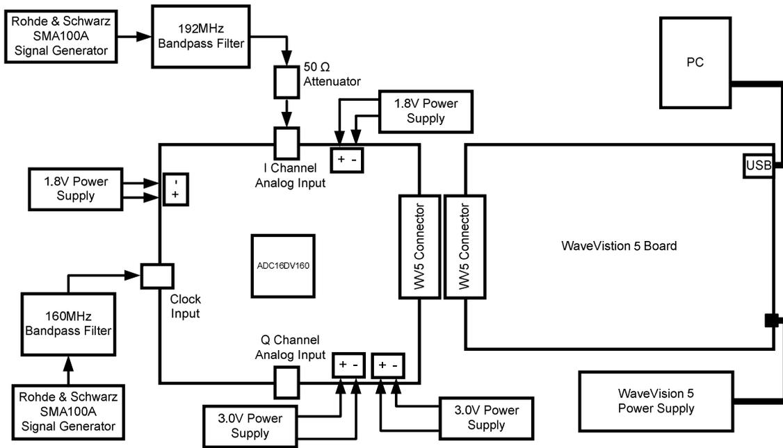
Figure 2: Test Set Up
