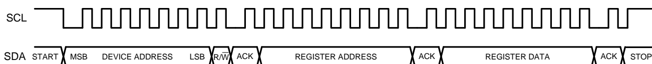
Figure 26. Example I 2 C Write Cycle
