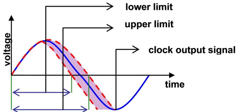
Figure 2-2. Window Trigger
