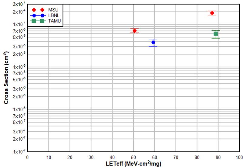
Figure 3-12. SEU Cross Section vs. LETeff with SYSREFOUT1 as Scope Trigger
