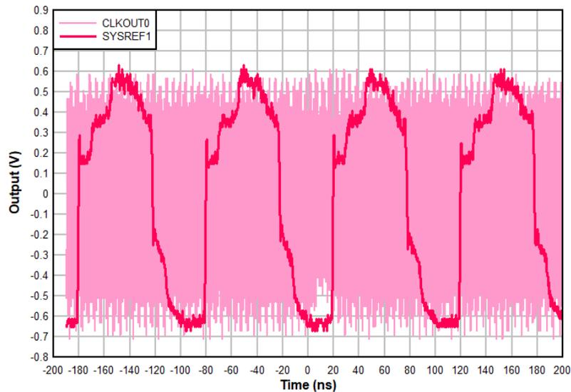
**Figure 3-9. Short SEU with SYSREF supplied directly from SYSREFREQ**
