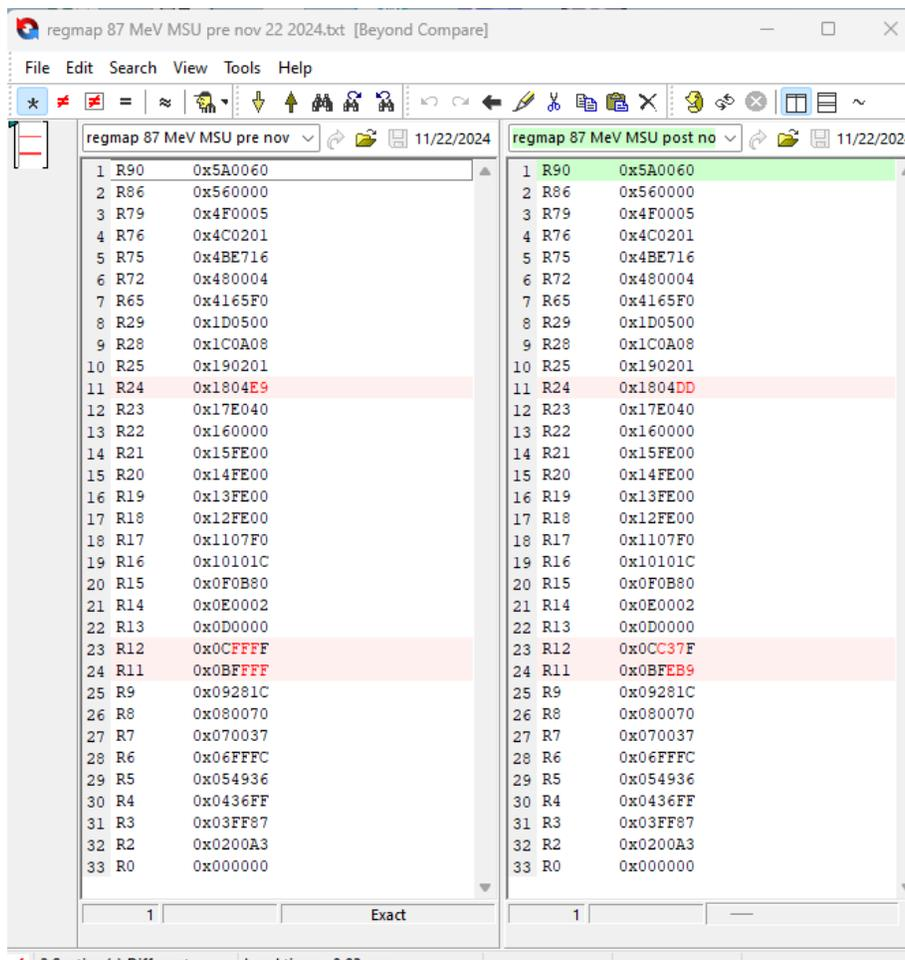
Figure 3-3. Screen Capture of Beyond Compare Comparing Registers Pre- and Post an Ion Run
