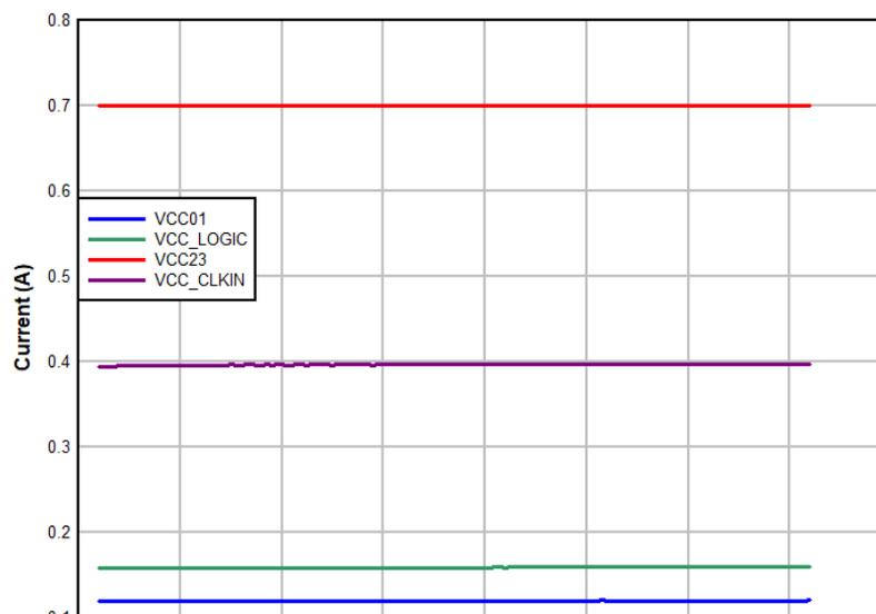
**Figure 3-1. Supply Currents During Ion Run 4 in Divide by 2 Mode**
