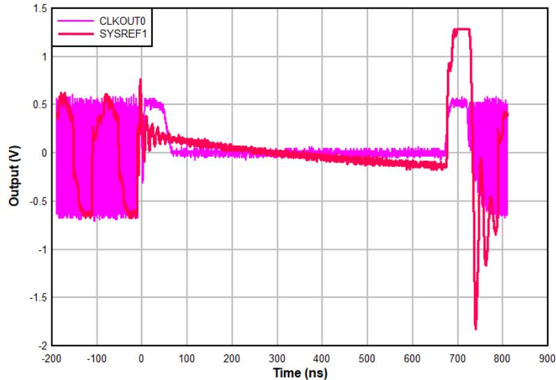
**Figure 3-8. Long SEU with SYSREF Supplied Directly from SYSREFREQ**
