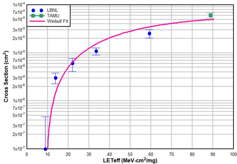
Figure 3-11. SEUs Cross Section vs. LETeff with CLKOUT0 as Scope Trigger
