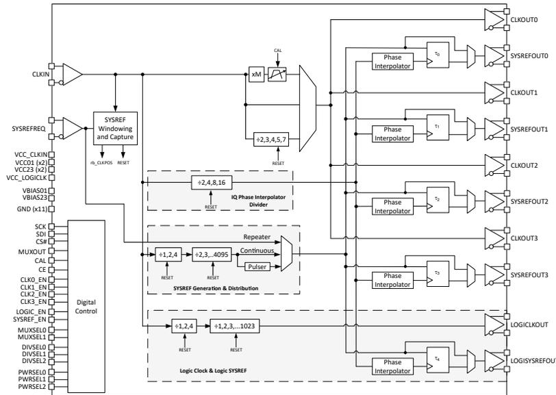
Figure 1-1. LMX1906-SP Block Diagram
