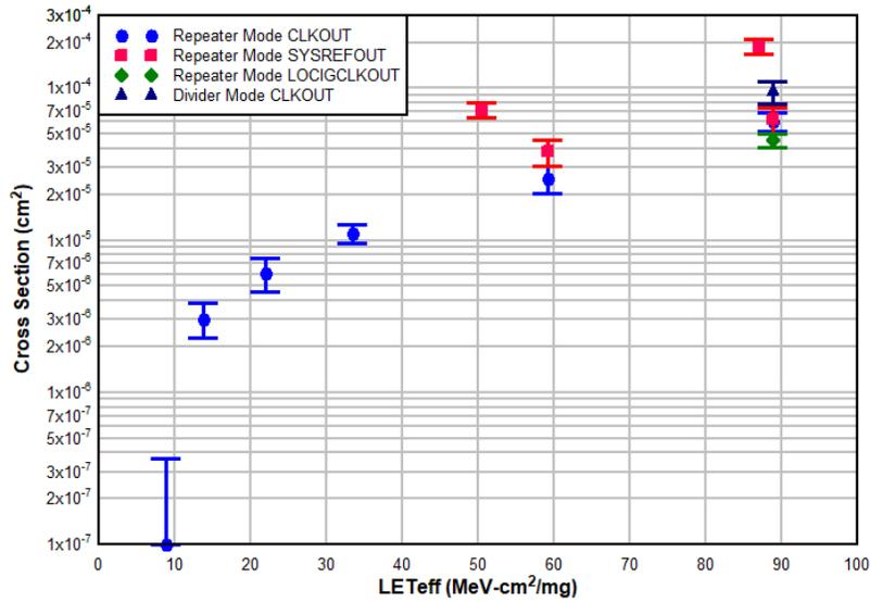
Figure 3-13. SEU Cross Section vs. LETeff for all Events with Operating Mode and Scope Trigger per the Legend
