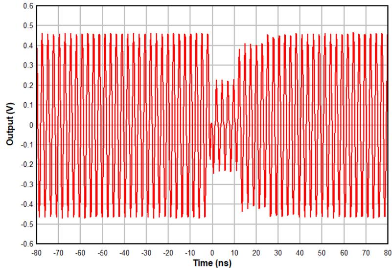
**Figure 3-7. SEU in Divider Mode with CLKOUT0 Recovering 180° Out of Phase**
