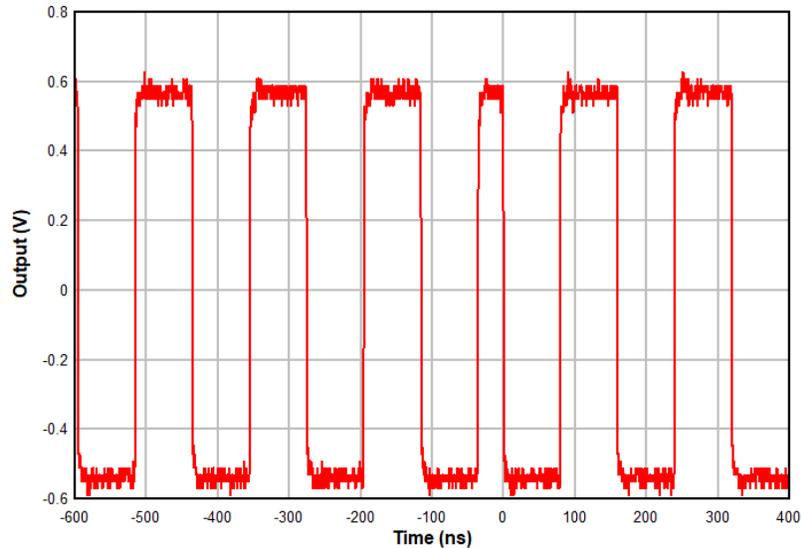
**Figure 3-6. SEU on SYSREFOUT1 where the Pulse Shortened**
