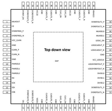
Figure 1-2. LMX1906-SP Pinout
