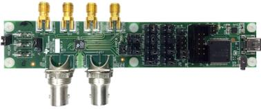
**LMH1297EVM: 12G Bidirectional I/O with Reclocker and Integrated Return Loss Network Evaluation Module**
