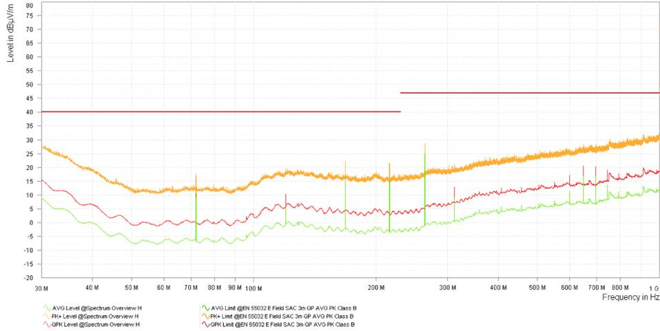
**Figure 3-7. Competitor C Quartz Oscillator**
