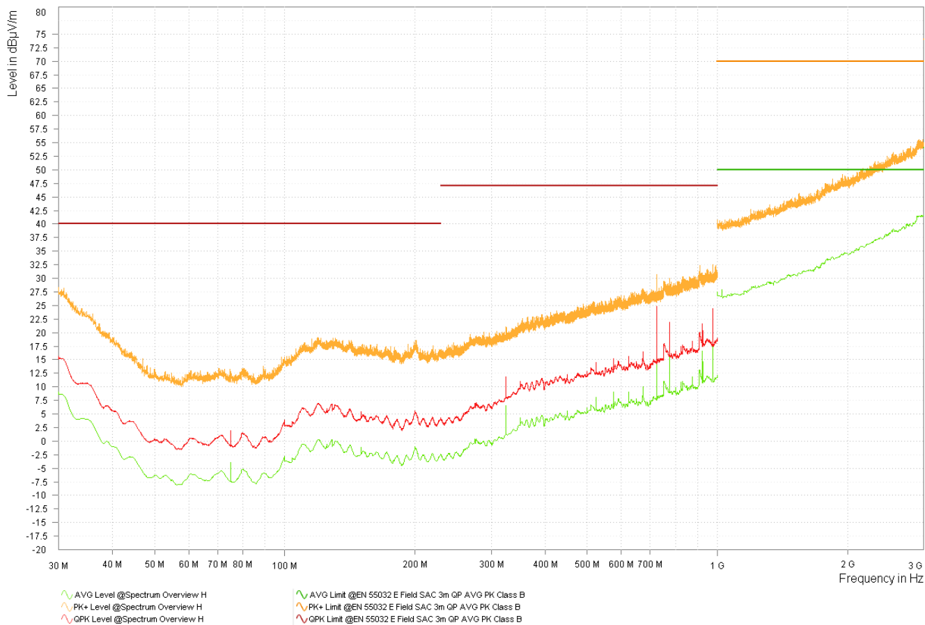
Figure 4-6. Variant 3 LMK3C0105 3.3V Y-Axis Spectrum Overview - Horizontal
