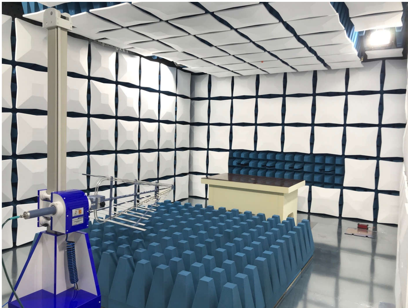
Figure 4-1. CISPR-32 Test Chamber Setup
