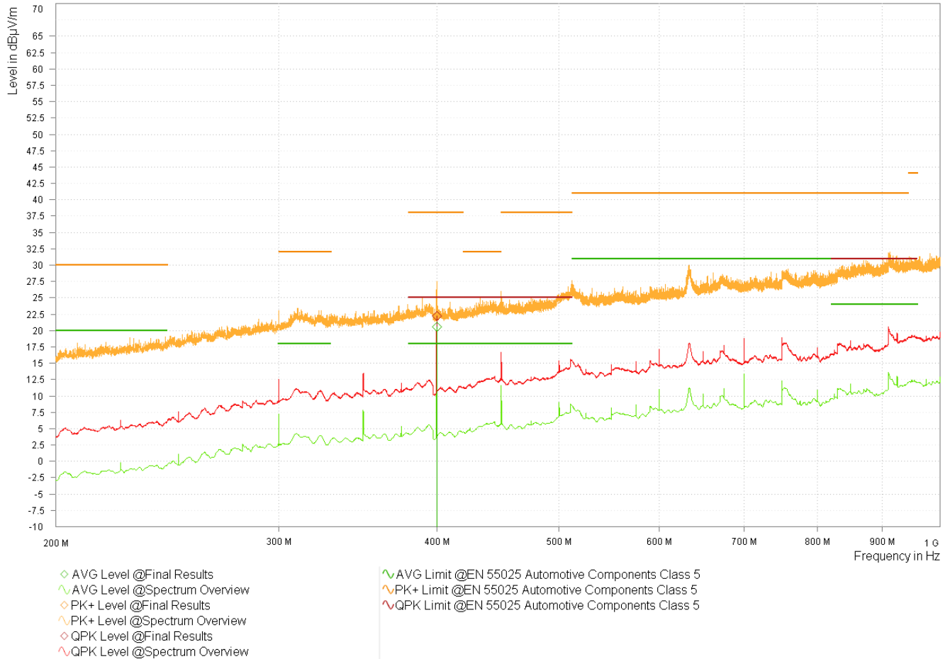
Figure 3-13. Variant 1 LMK3C0105 3.3V Spectrum Overview - Log-Periodic
