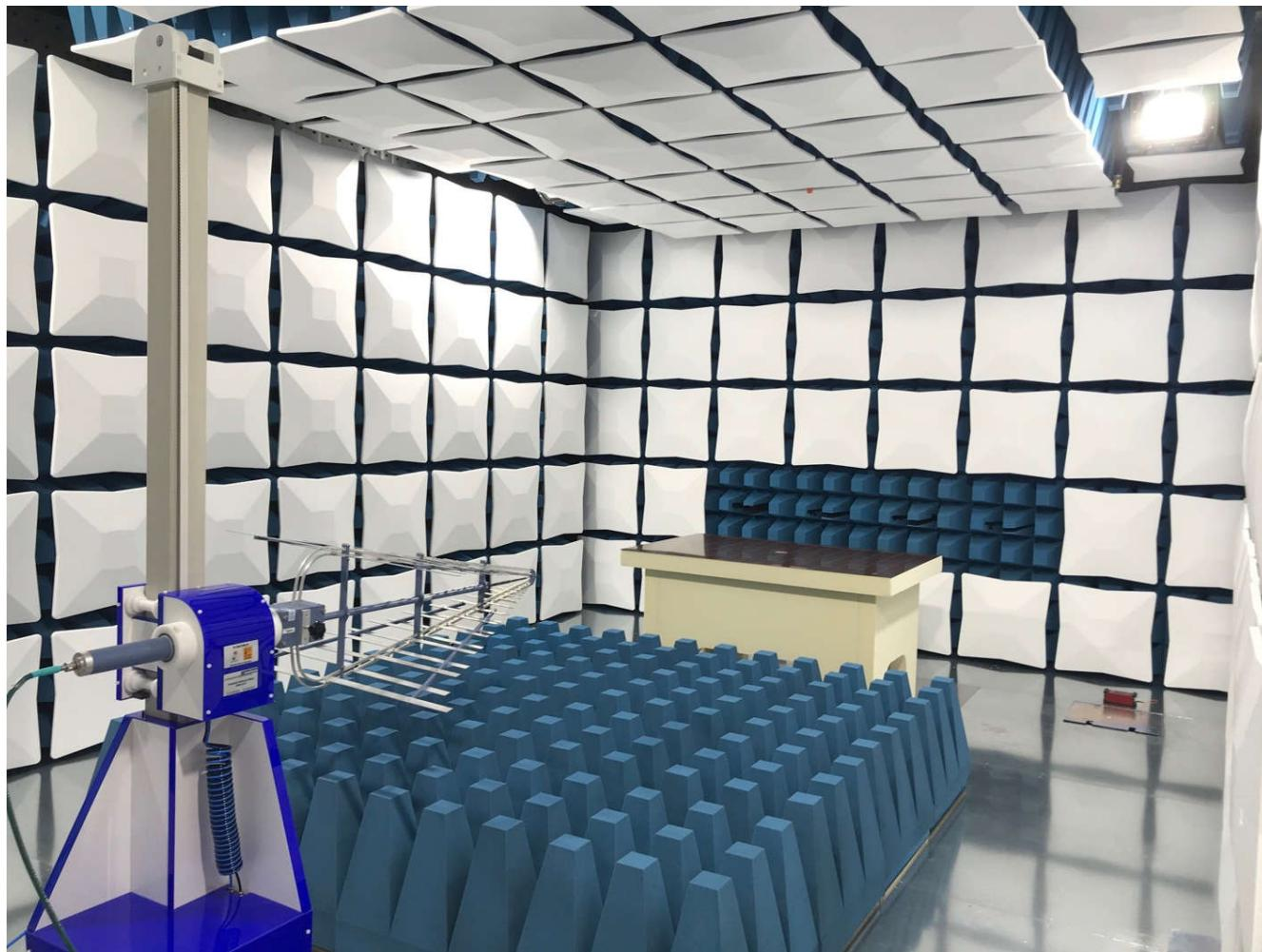
Figure 4-1. CISPR-32 Test Chamber Setup
