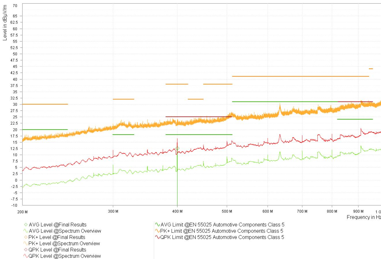
**Figure 3-14. Variant 2 LMK3C0105-Q1 3.3V Spectrum Overview - Log-Periodic**
