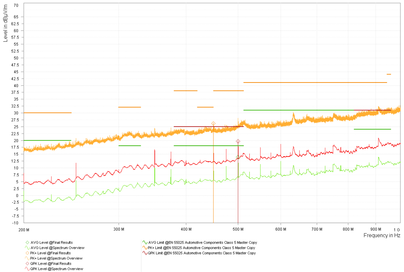
Figure 3-19. Competitor Oscillator 3.3V Spectrum Overview - Log-Periodic
