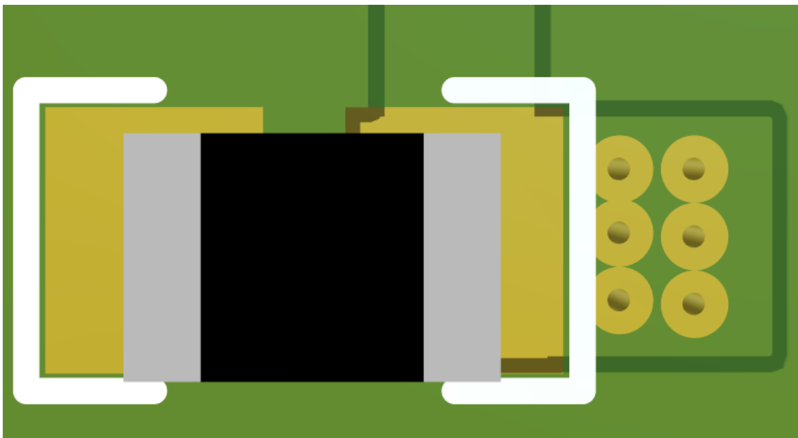
Figure 3-9. Large Passive with Many Vias
