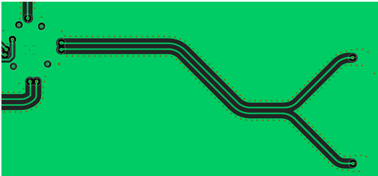
Figure 3-12. Clock Traces with Shielding Vias
