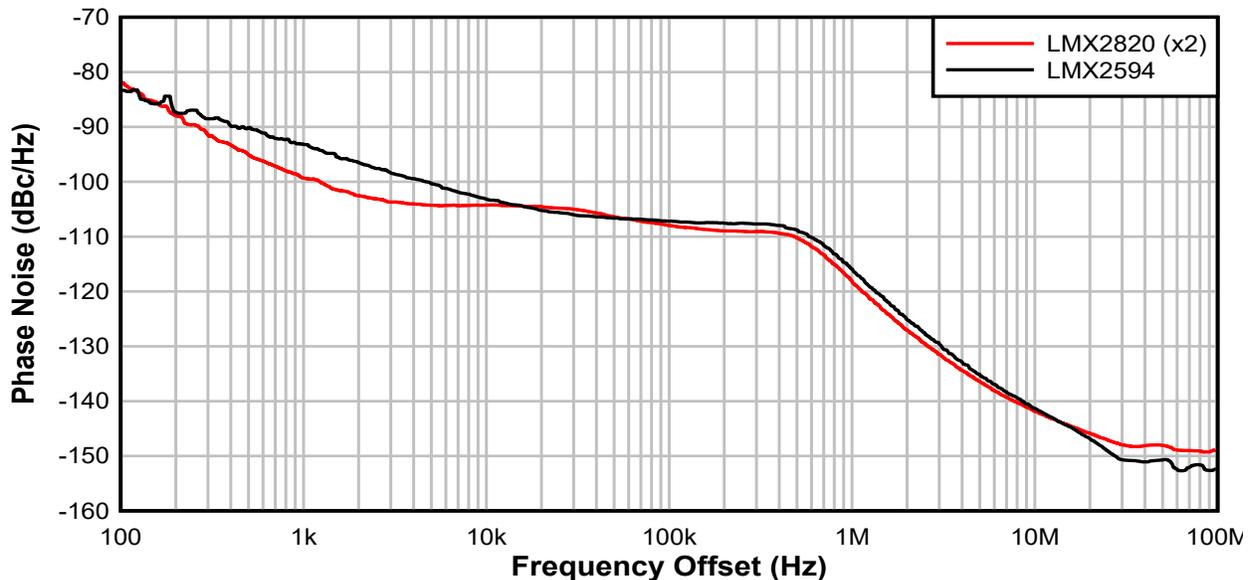
Figure 1-1. Phase Noise Comparison of LMX2594 vs LMX2820 with Internal Doubler at 13.2GHz
