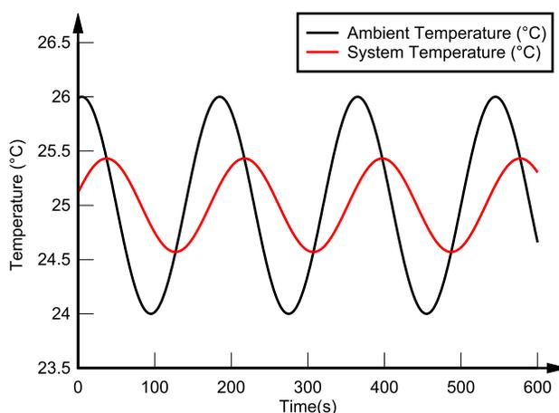
**Figure 4-4. Simulated System Thermal Response ( $\tau = 60s$ ) to a Temperature Cycling Ambient Environment**
