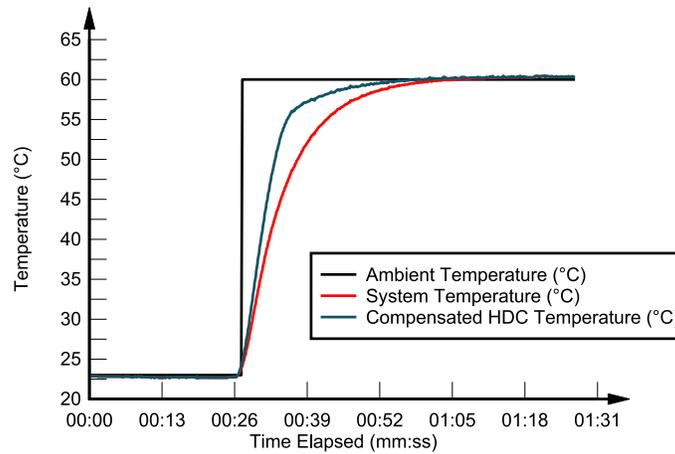
**Figure 4-13. Compensated System Response to Ambient Temperature Change from Room (~23 °C) to 60 °C, with k=50**
