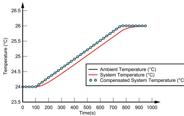
Figure 4-7. Compensated System Temperature Response (Blue) to a Ramp Change in Temperature
