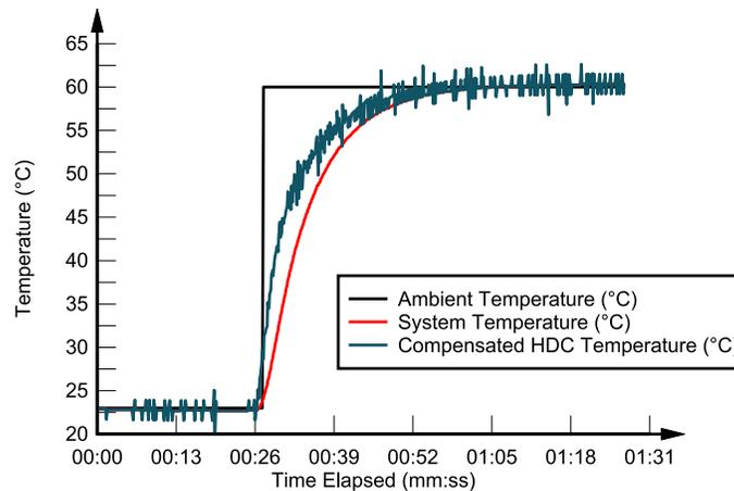
**Figure 4-10. Compensated System Response to Ambient Temperature Change From Room (~23 °C) to 60 °C,  $\tau \approx 9.1s$**
