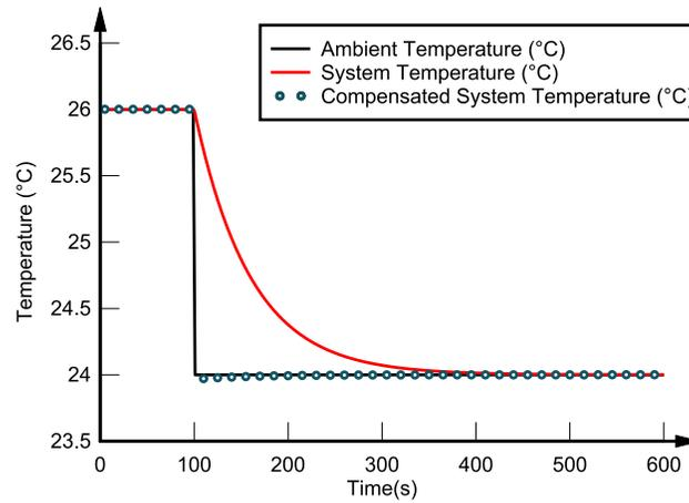
Figure 4-6. Compensated System Temperature Response (Blue) to a Step Change in Temperature
