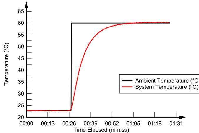
**Figure 4-9. System Response to Ambient Temperature Change from Room (~23 °C) to 60 °C,  $\tau \approx 9.1s$**
