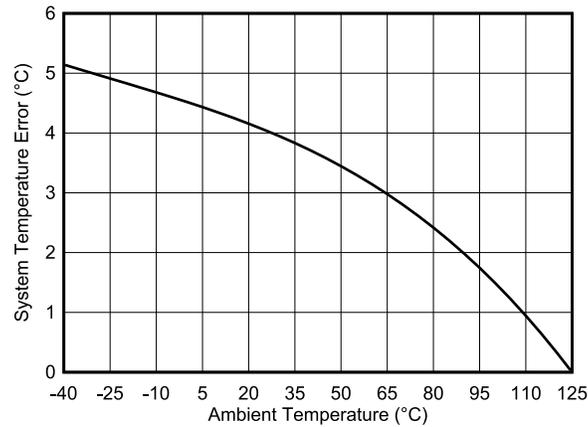
Figure 2-1. System Temperature Error Across Ambient Temperature
