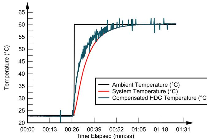
**Figure 4-11. Compensated System Response to Ambient Temperature Change from Room (~23 °C) to 60 °C, Including Threshold triggered predictive response**
