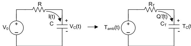
**Figure 4-2. Typical RC Circuit and its Thermal Analogue**
