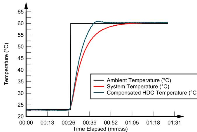
**Figure 4-14. Compensated System Response to Ambient Temperature Change From Room (~23 °C) to 60 °C, with k=100**
