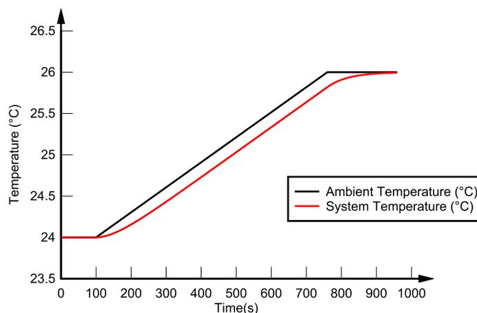
**Figure 4-3. Simulated System Thermal Response ( $\tau = 60s$ ) to a Steady Change in Temperature**
