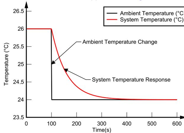
**Figure 4-1. Simulated System Thermal Response ( $\tau = 60s$ ) to a Step Change in Temperature**
