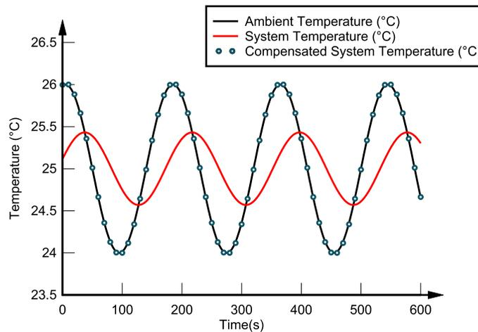
Figure 4-8. Compensated System Temperature Response (Blue) for a Temperature Cycling Ambient Environment
