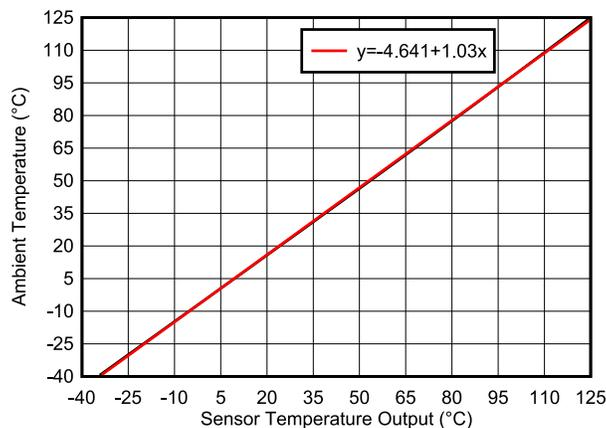
Figure 2-2. Ambient Temperature as a Function of Sensor Output Temperature
