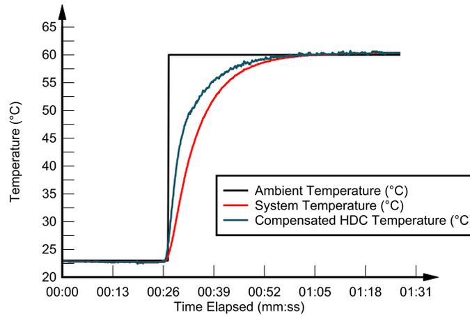
**Figure 4-12. Compensated System Response to Ambient Temperature Change from Room (~23 °C) to 60 °C, with k=10**
