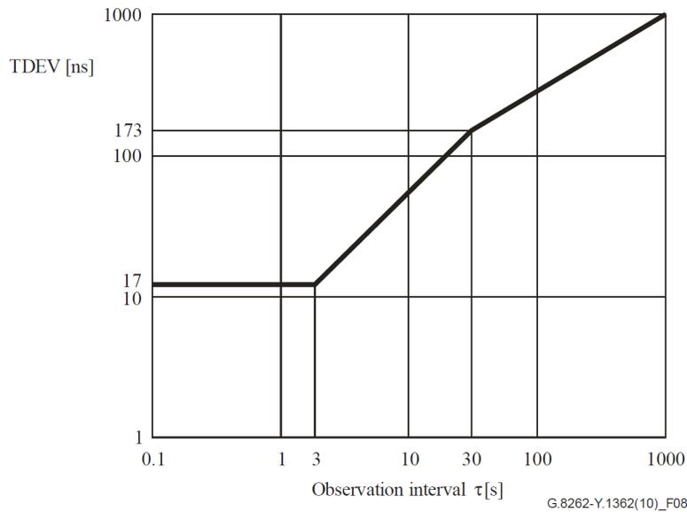
Figure 19. Input Wander Tolerance (TDEV) for EEC-Option 2
