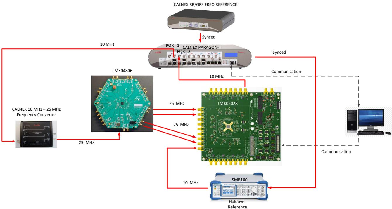
**Figure 23. Test Setup for Phase Transient Generation**
