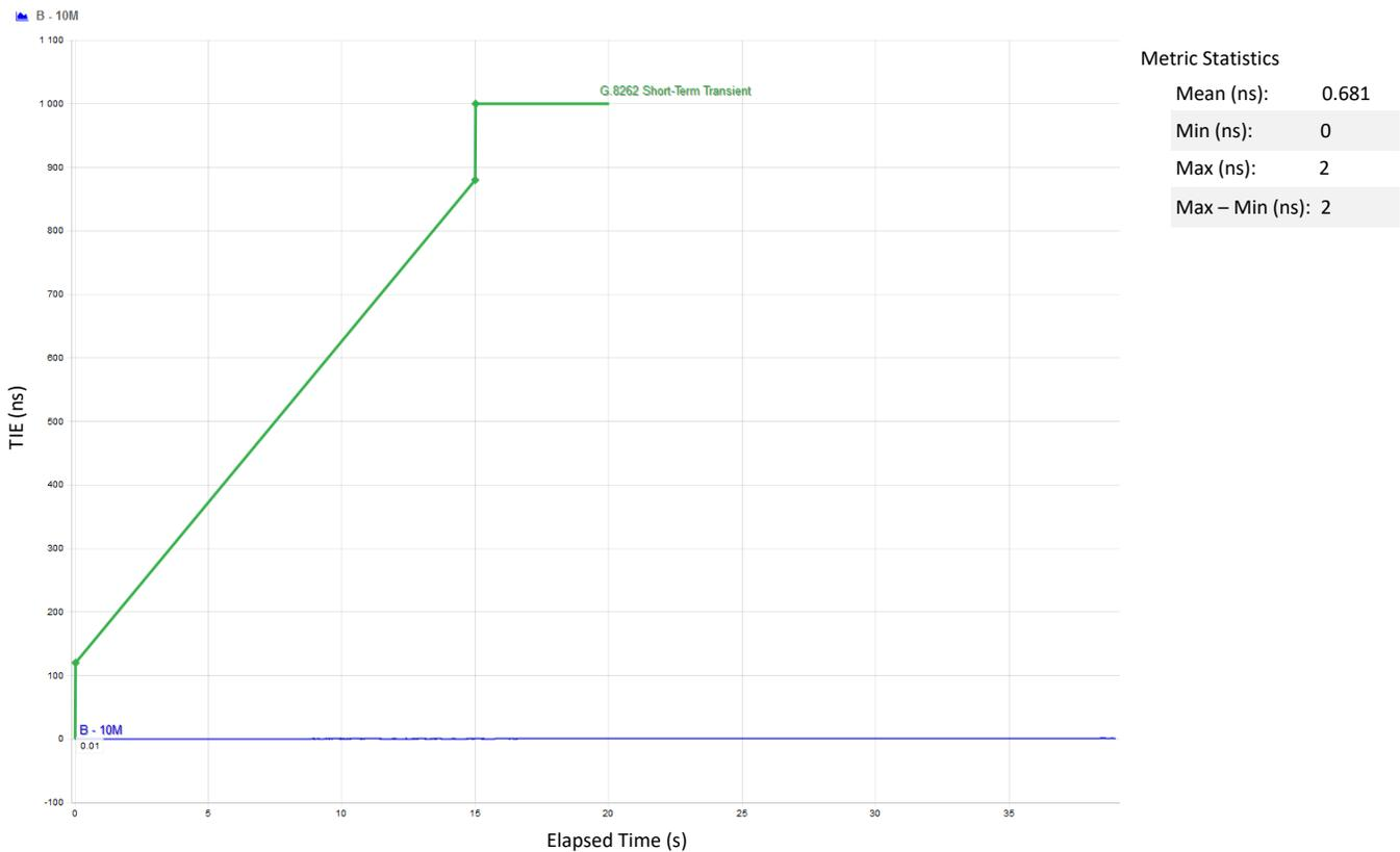
**Figure 29. Phase Transient With Signal Interruptions Results**
