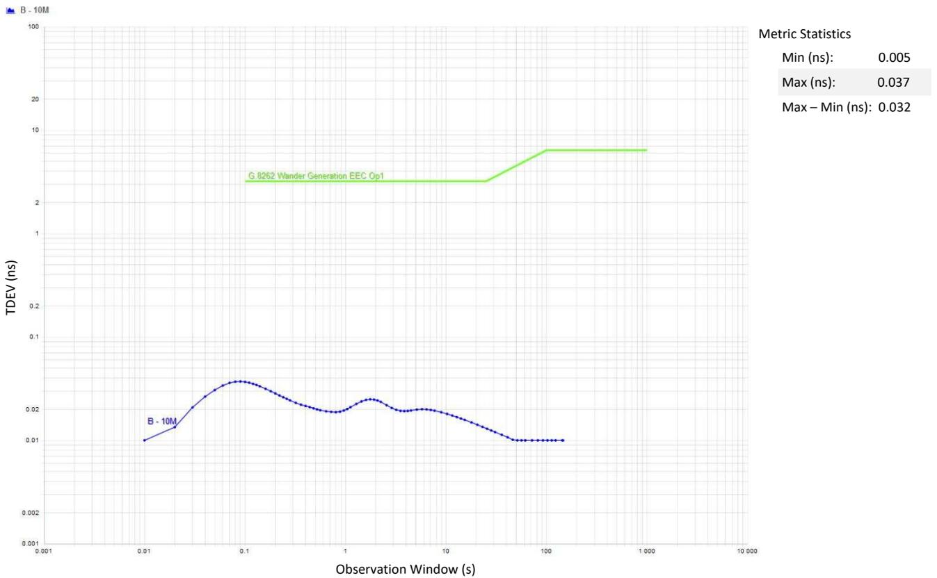
Figure 6. Wander Generation TDEV G.8262 EEC Option 1 Results, Tested at Constant Room Temperature With DPLL Bandwidth of 5 Hz
