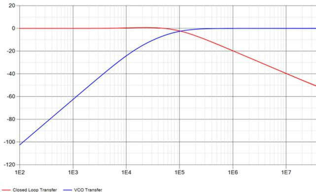
Figure 44. PLL Closed-Loop Response With 3rd Order Pole
