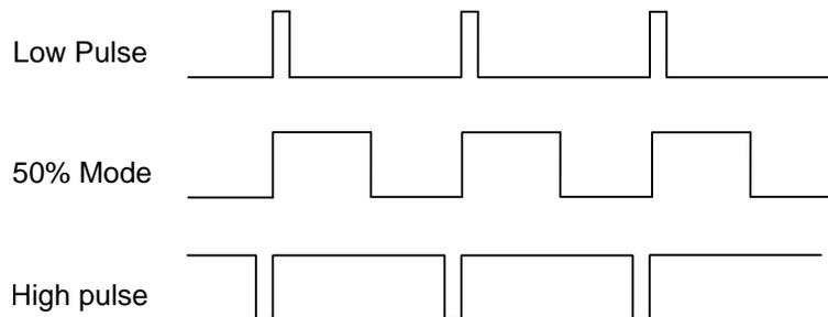
**Figure 6. Three Mode Options Supported by the LMK046xx**
