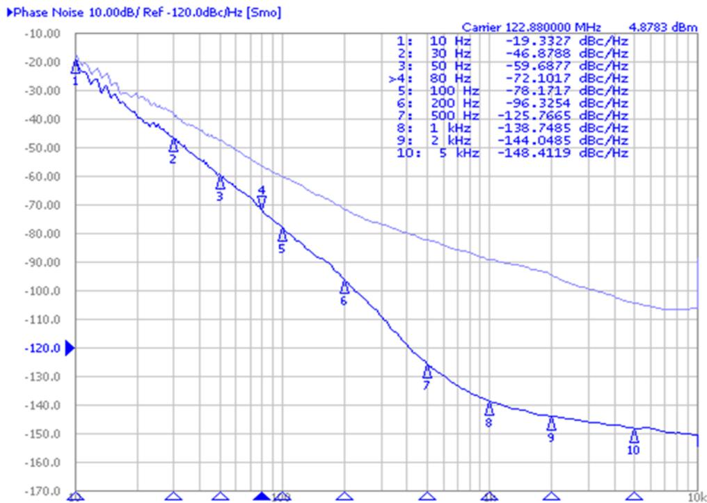
Figure 29. Output Clock Phase Noise With CCTRL = 4.7 µF
