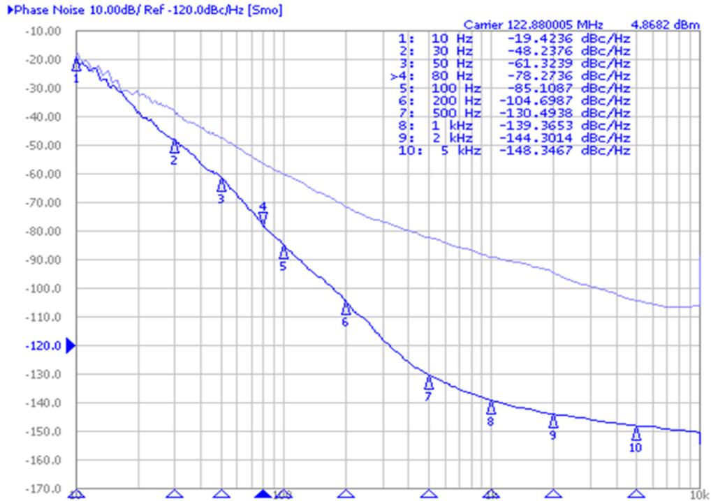
Figure 30. Output Clock Phase Noise With CCTRL = 10 µF
