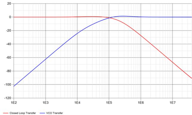
Figure 45. PLL Closed-Loop Response Without 3rd Order Pole
