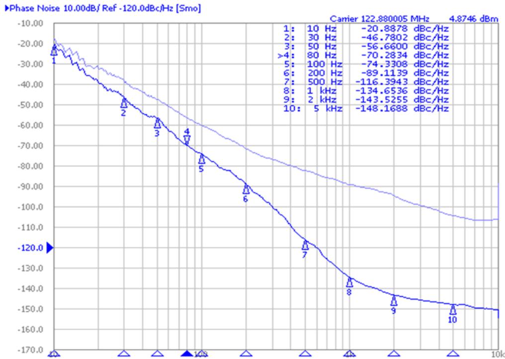
Figure 28. Output Clock Phase Noise With CCTRL = 1 µF
