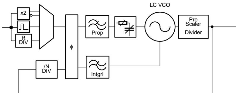
Figure 33. PLL2 Block Diagram
