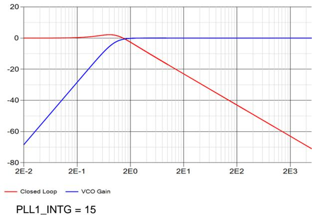
Figure 19. PLL1 Closed-Loop Response
