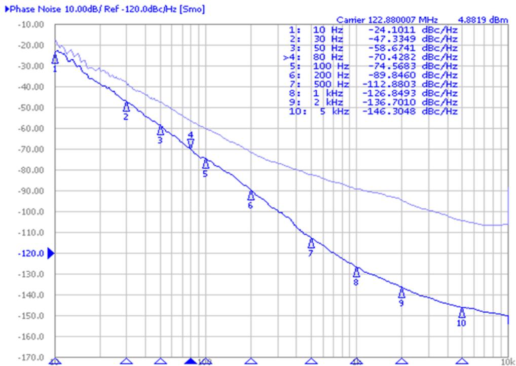
Figure 27. Output Clock Phase Noise With CCTRL = 200 nF
