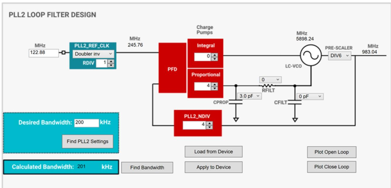
Figure 35. TICSPRO PLL2 Loop Filter Design Tool
