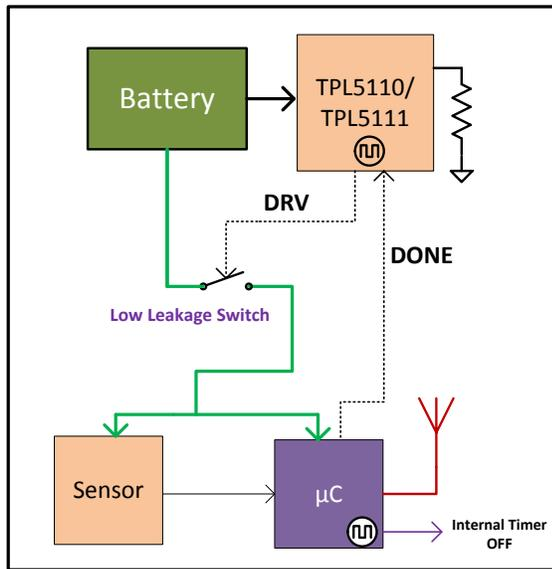
**Figure 2. A Sensor Node with an Integrated Power-gating System Nanotimer**
