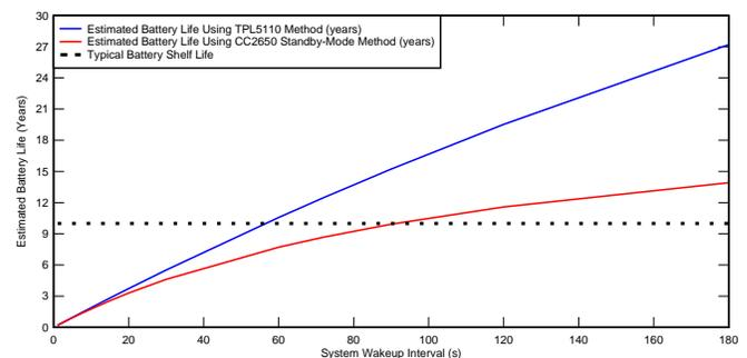
**Figure 4. Estimated Battery Life Comparison: Nanotimer vs. MCU Standby Mode**
