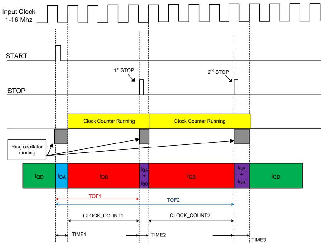
**Figure 4. Measurement Mode 2**
