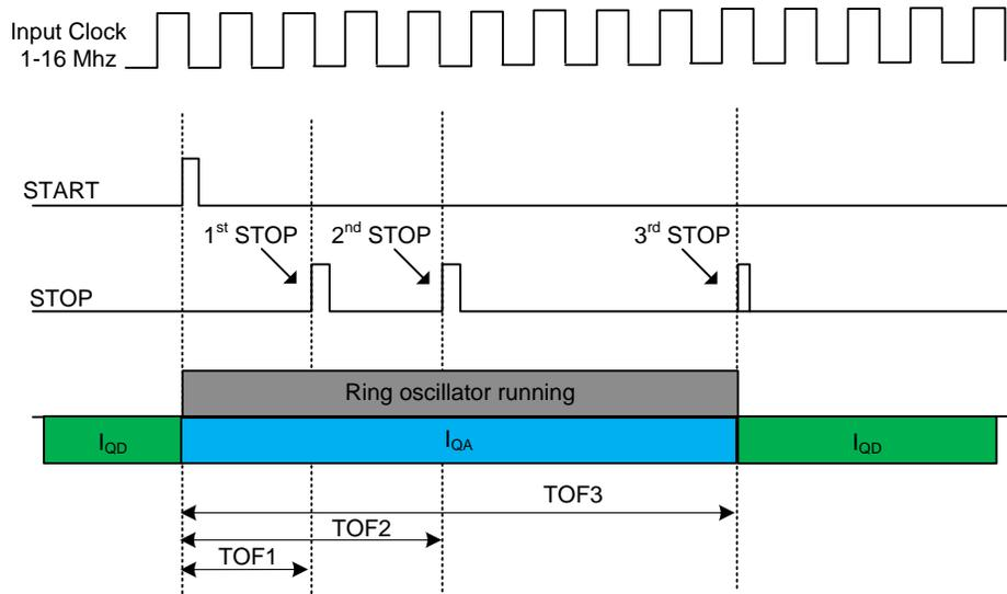
**Figure 3. Measurement Mode 1**
