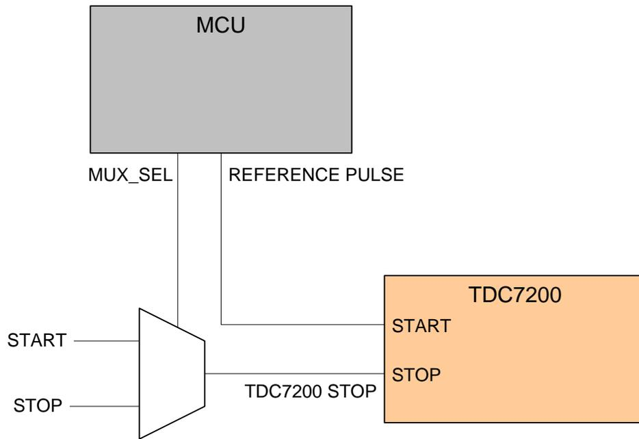
Figure 5. Interleaved Short Time Measurements Block Diagram
