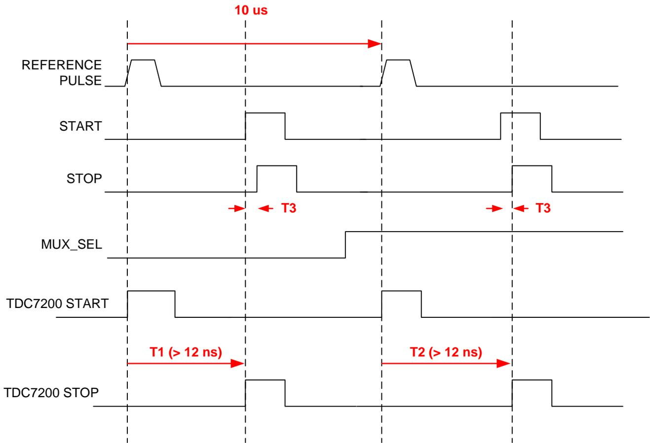
Figure 6. Interleaved Short Time Measurements Timing Diagram
