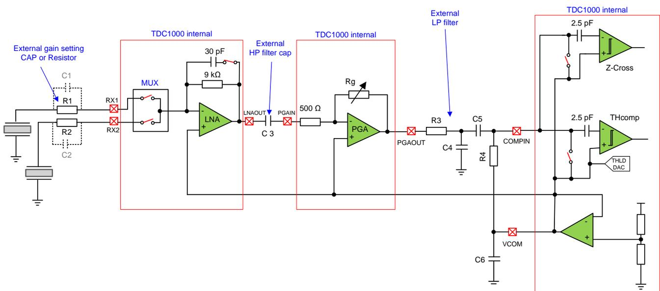
Figure 5. Simplified Diagram of the TDC1000 Receiver Path
