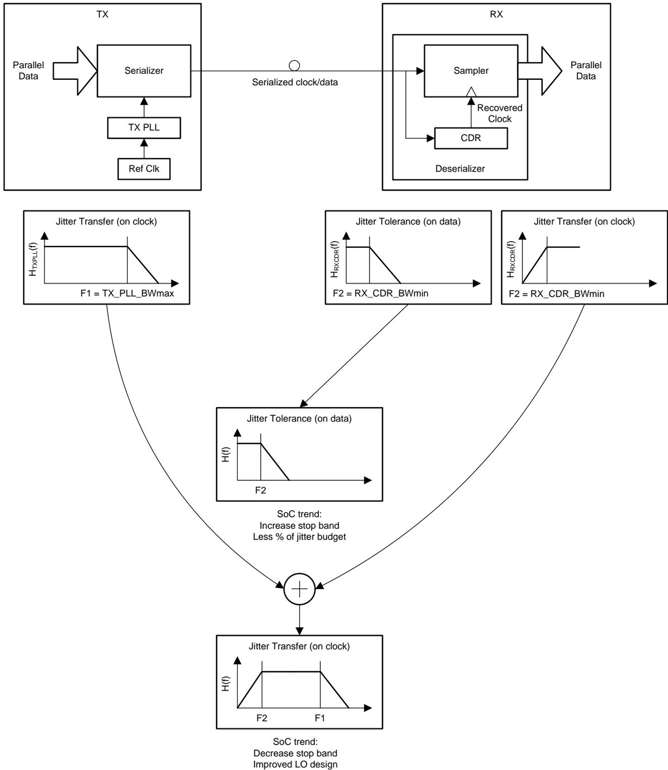
Figure 1. Dependence of Clock Jitter in Serial Links
