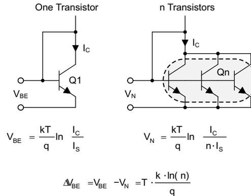
Figure 5. Principle of Eliminating  $I_C$  and  $I_S$
