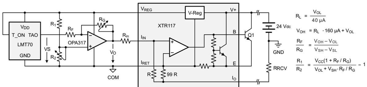
Figure 15. Low-Cost Temperature Transmitter With 4-to-20 mA Output
