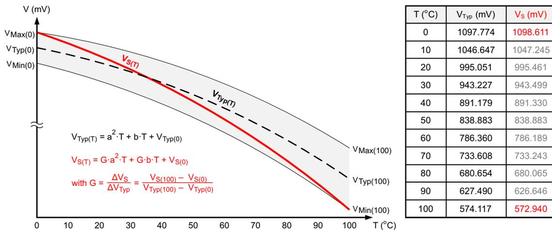
Figure 11. Sensor Output Characteristic Versus Typical Characteristic
