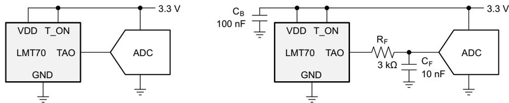
**Figure 9. Circuit Examples for Noise-Free and Noisy Environments**
