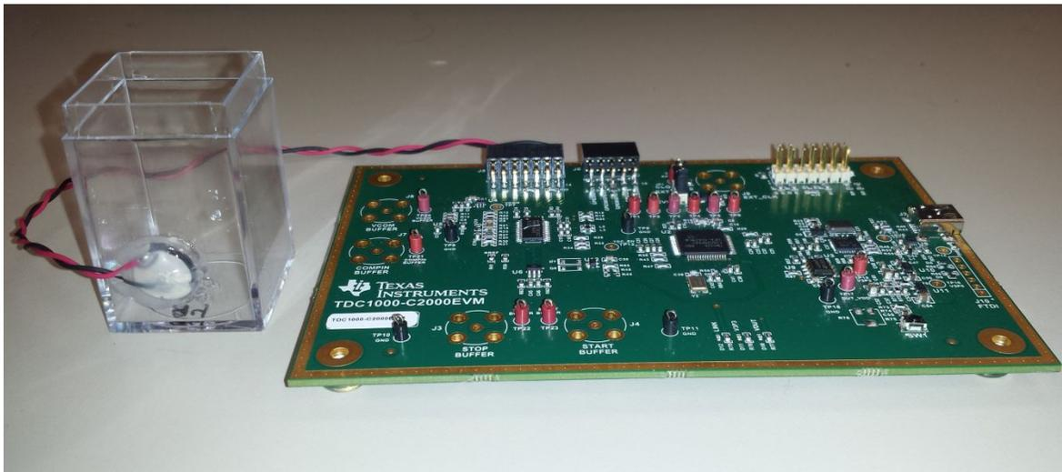
Figure 2. TDC1000-C2000 EVM with Test Cell
