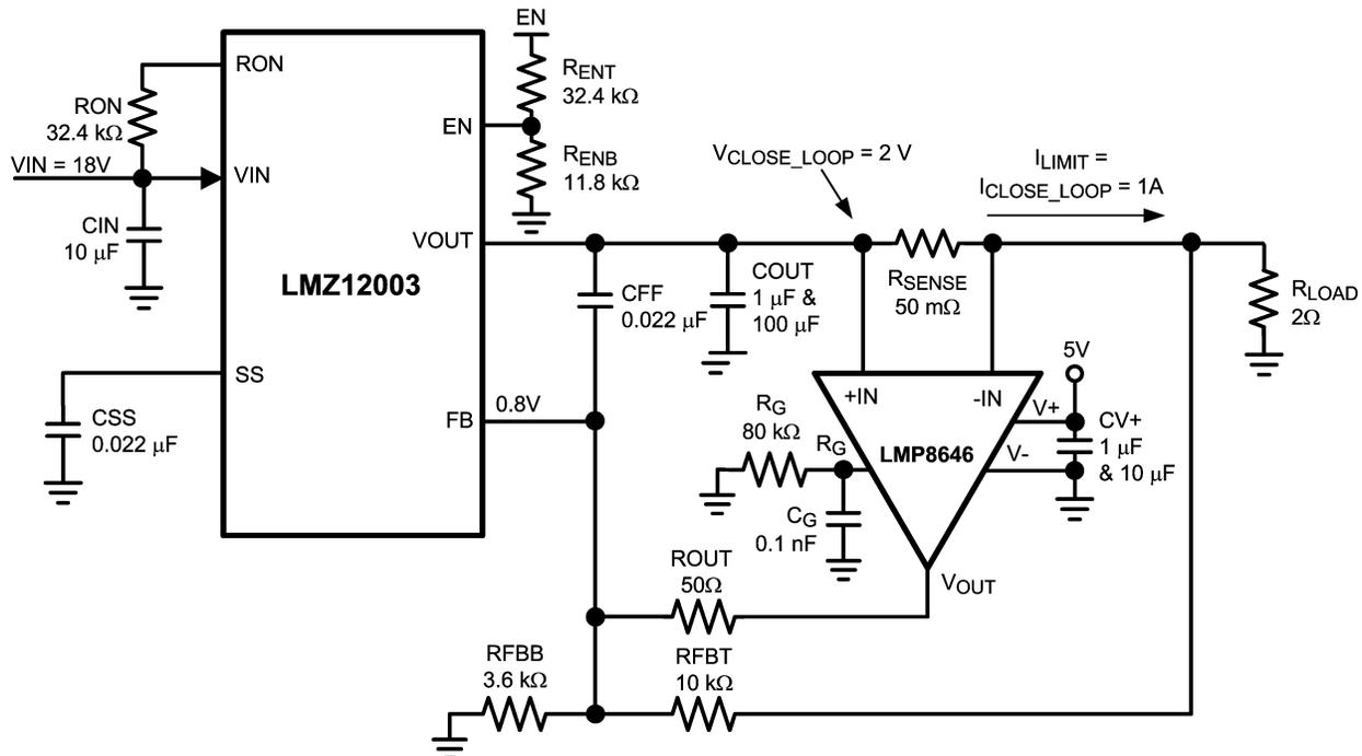
**Figure 1. Resistive Load Application with LMZ12003 Regulator and LMP8646 Precision Current Limiter**
