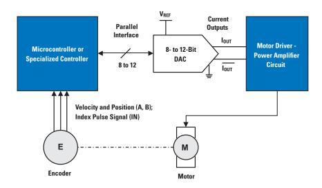
Figure 3. Motor Control Example
