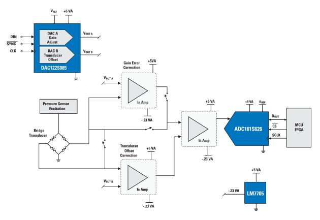
Figure 2. Simplified Example of a Calibrated Pressure Sensing Diagram
