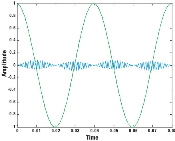
**Figure 5. Error Signal Due to Time Skew between Interleaved ADC Clocks, M=4**
