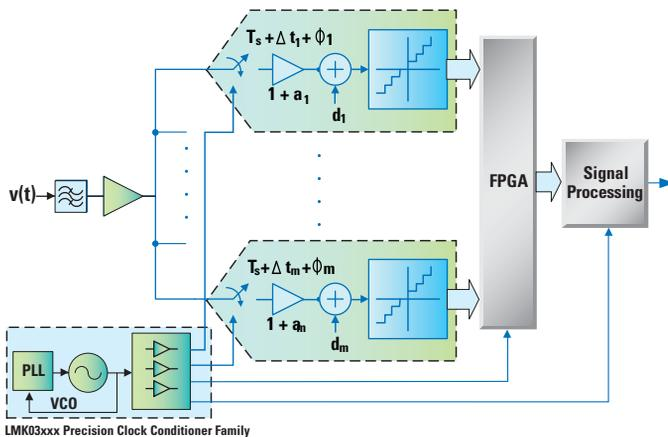
**Figure 3. ADC Model with DC, Gain, and Time Skew Offsets**
