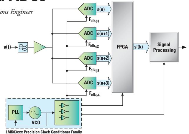
Figure 1. Time-Interleaved ADC System
