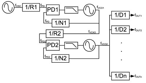
Figure 9. Dual Loop Architecture
