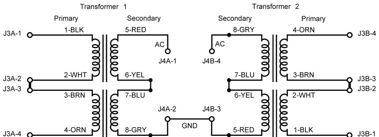
**Figure 3. 240V Transformer Connections, Primaries in Series**
