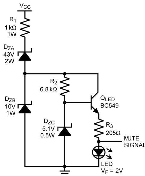
Figure 10. Constant Brightness LED and Mute Control Circuit
