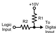
**Figure 3. Simple Digital Input Level Shifting Circuit**
