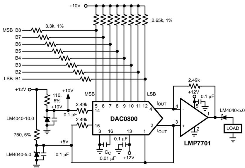
Figure 5. Complete Single Supply DAC0800 Design With 0 V to 5 V Output
