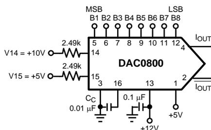
**Figure 2. Positive Only Supply Circuit for the DAC0800**
