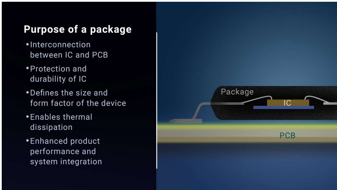
Figure 1. Internal diagram of a typical analog package, and what packaging accomplishes.
