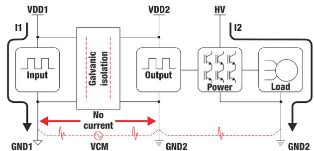
**Figure 1.** Low- to high-voltage galvanic signal isolation.
