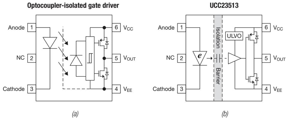
**Figure 3.** Comparison of optocoupler-isolated gate driver (a) and capacitively isolated gate driver (b).
