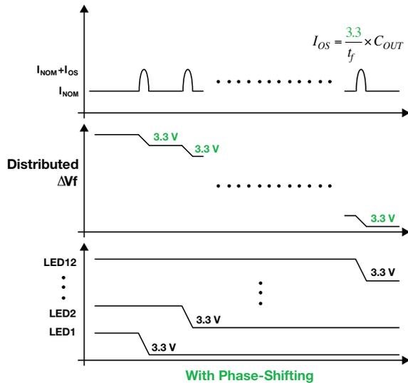
**Figure 4.** Phase-shifted turnoff of 12 LEDs on an LMM.
