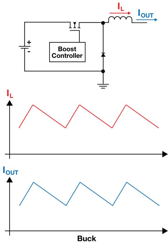
Figure 6. Output current of a buck converter.
