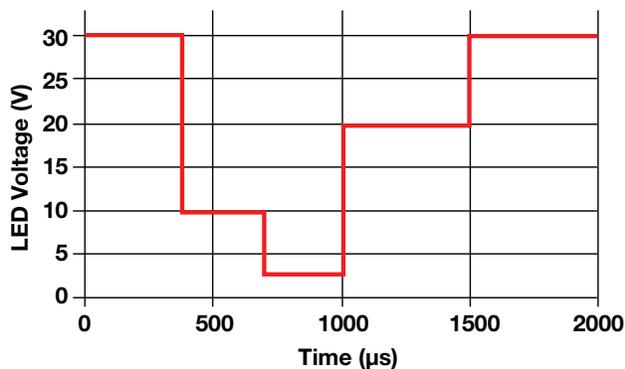
**Figure 2.** Variation of LED voltage (dynamic LED load).
