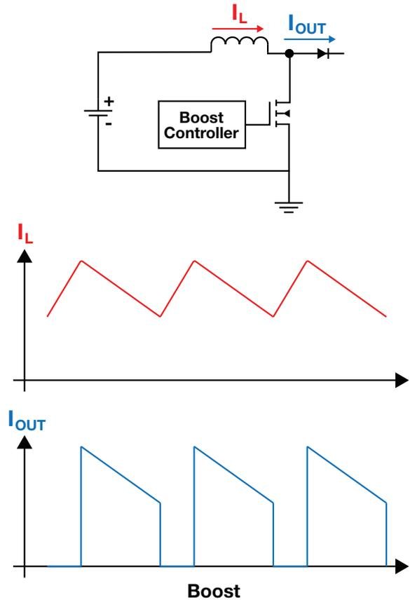
**Figure 5.** Output current of a boost converter.
