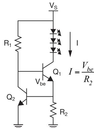
**Figure 8.** A current-source LED circuit with two transistors.
