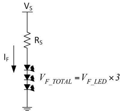
**Figure 4.** Direct LED drive with  $R_S$ .
