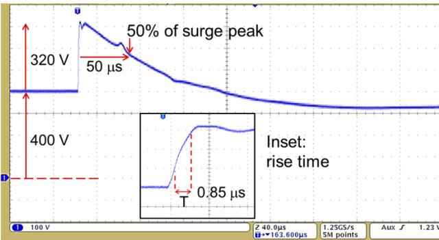
Fig. 7: Measurement of the open-circuit surge waveform for a 720 V peak output with 400 V DC component. The front time is 1.42  $\mu$ s and duration is 50  $\mu$ s, in accordance with the IEC 61000-4-5 definitions in Fig. 1.
