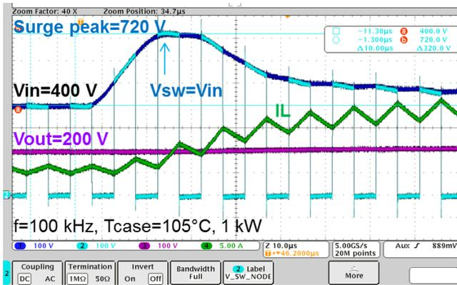
Fig. 6: Surge waveforms, showing the test-point parameters labeled in Fig. 4. The input bus voltage surges from the operating point of 400 V to the target spec of 720 V. The switched node waveform is overlaid on the input waveform to show the switching. It shows that the 720 V surge stress is applied directly to the GaN FETs while switching.
