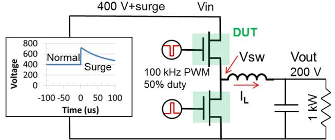
Fig. 4: Surge test-vehicle schematic topology. The circuit biases the device at a 400 V operating point and applies surges while the devices are actively running, in order to replicate the real operating condition of a surge.
