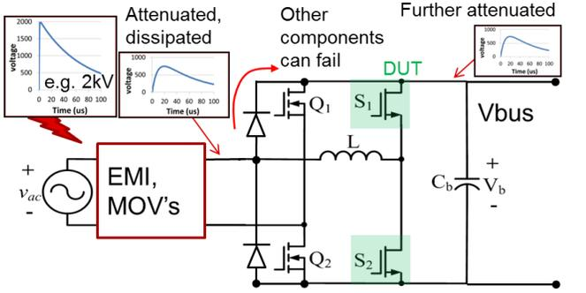
Fig. 2: Schematic of a PFC stage, showing the attenuation of the waveform and the system-dependence of the surge voltage reaching the device.
