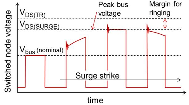
Fig. 3: Figure illustrating the two datasheet parametrics needed to fully surge-rate a device:  $V_{DS(SURGE)}$ , the maximum bus voltage allowable during surge, and  $V_{DS(TR)}$ , to specify additional headroom for ringing.
