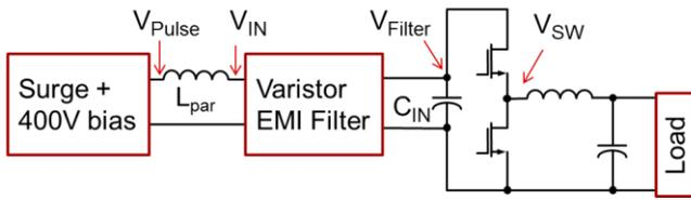
Fig. 9: Schematic of the buck converter used for simulation
