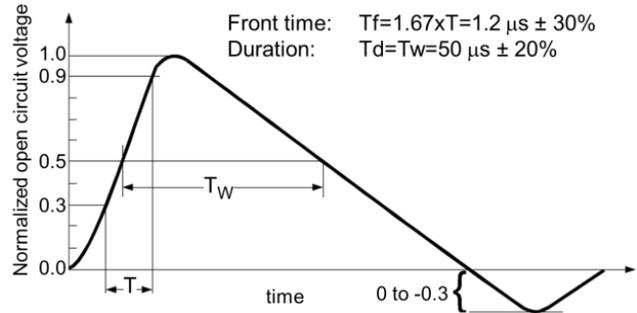
Fig. 1: IEC 61000-4-5 standard CWG 1.2/50  $\mu$ s open-circuit surge waveform shape to simulate a line disturbance. The front time is 1.2  $\mu$ s, and duration (above 50% of the peak value) is 50  $\mu$ s.
