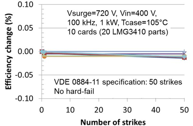
Fig. 8: The 50-strike surge test, validating that devices do not show efficiency degradation or hard-failure, and continue to power a 1 kW load.
