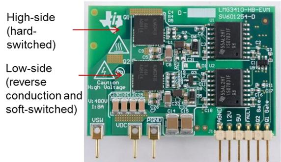
Fig. 5: TI-GaN EVM half-bridge card used for the device test. It plugs into the surge-tester motherboard. The use of a half-bridge allows surge testing for both polarities: hard-switching turn-on and reverse conduction.
