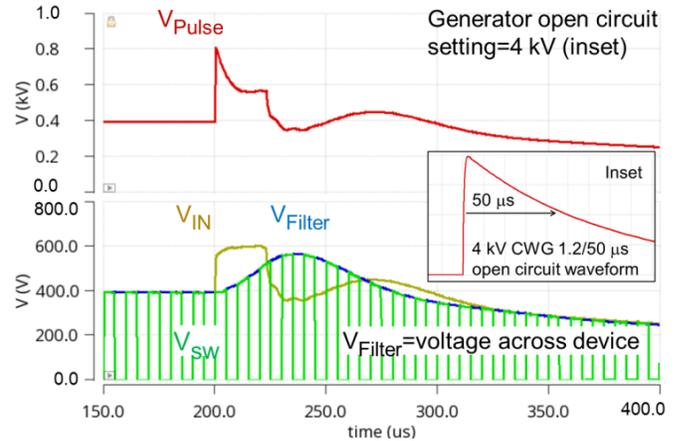
Fig. 10: Simulation of a 4kV surge setting applied to a power supply. The peak device voltage is less than 570V, well below the device surge rating. This illustrates the design of a surge-robust GaN power supply.
