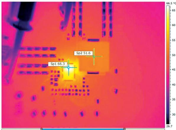
Figure 5. TPS548B22 thermal performance,  $T_{max} = 66.3^{\circ}\text{C}$ .
