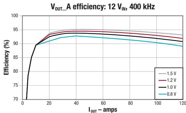
**Figure 9.** TPSM831D31 module channel at 120-A efficiency.
