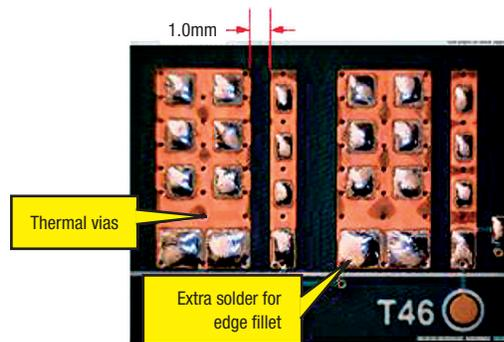
Figure 2. TPSM831D31 PCB bottom pads – all rectangles.
