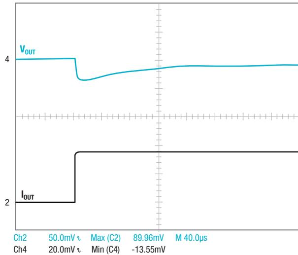
**Figure 12.** TPSM831D31 load transient – 30-A step, 100 A/µs.
