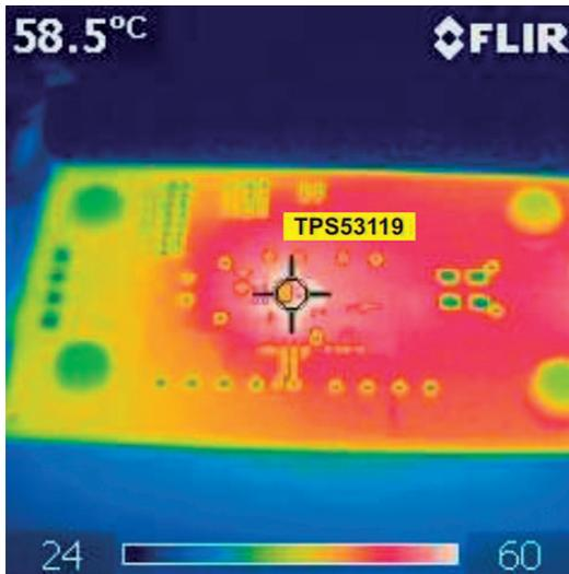
Figure 4. TPS53119 thermal performance,  $T_{max} = 58.5^{\circ}\text{C}$ .
