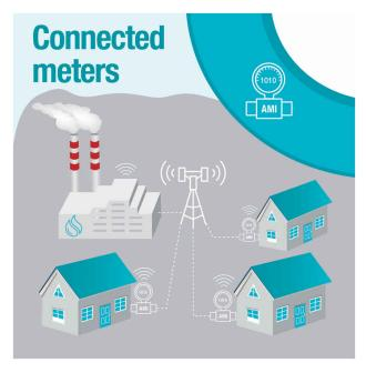
Although connected meter deployments initially started with electricity, the adoption of automatic meter reading (AMR) and smart meters within the flow meter market (gas, water, heat) is also gaining momentum.
