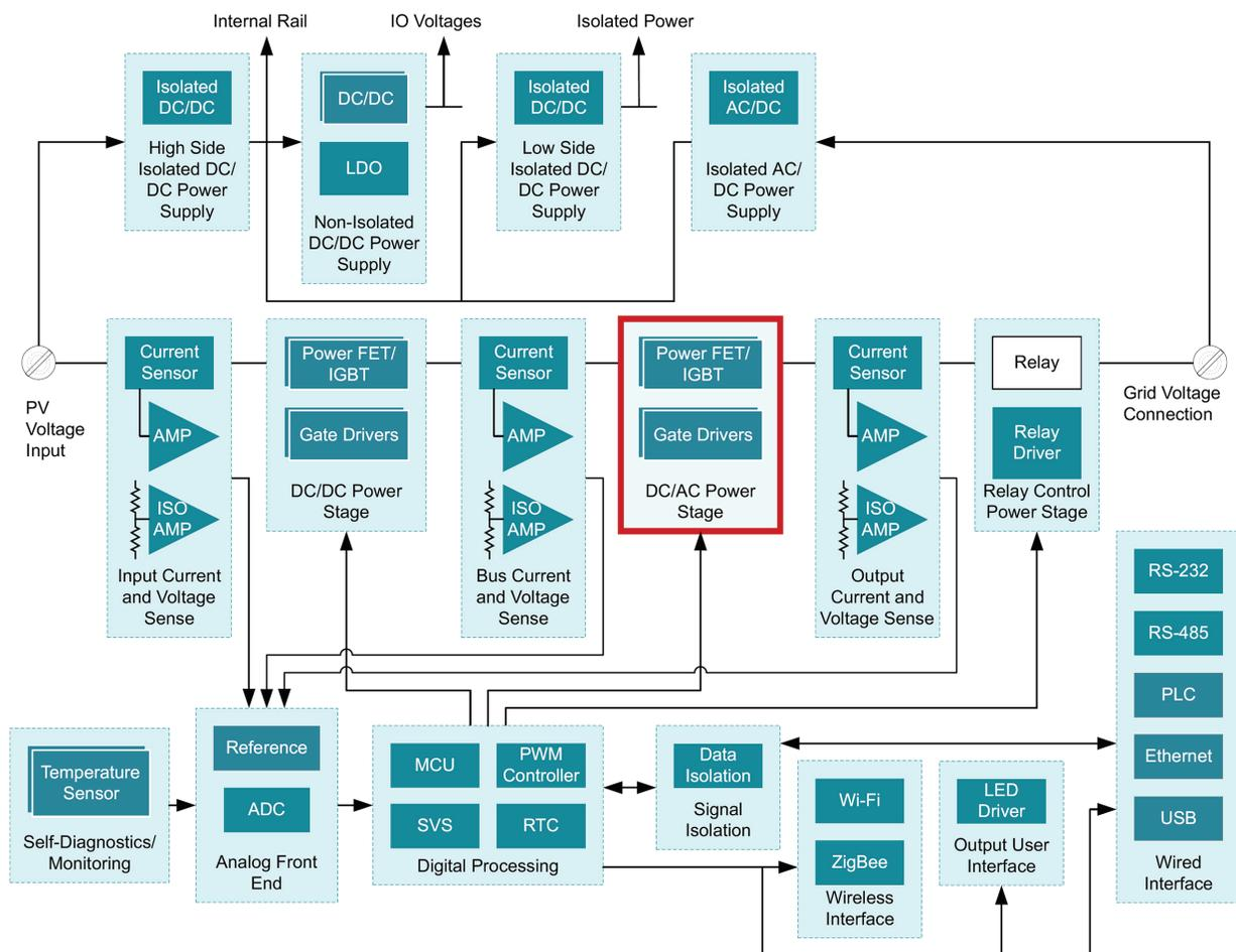
**Figure 2.** . Block diagram of a string inverter.
