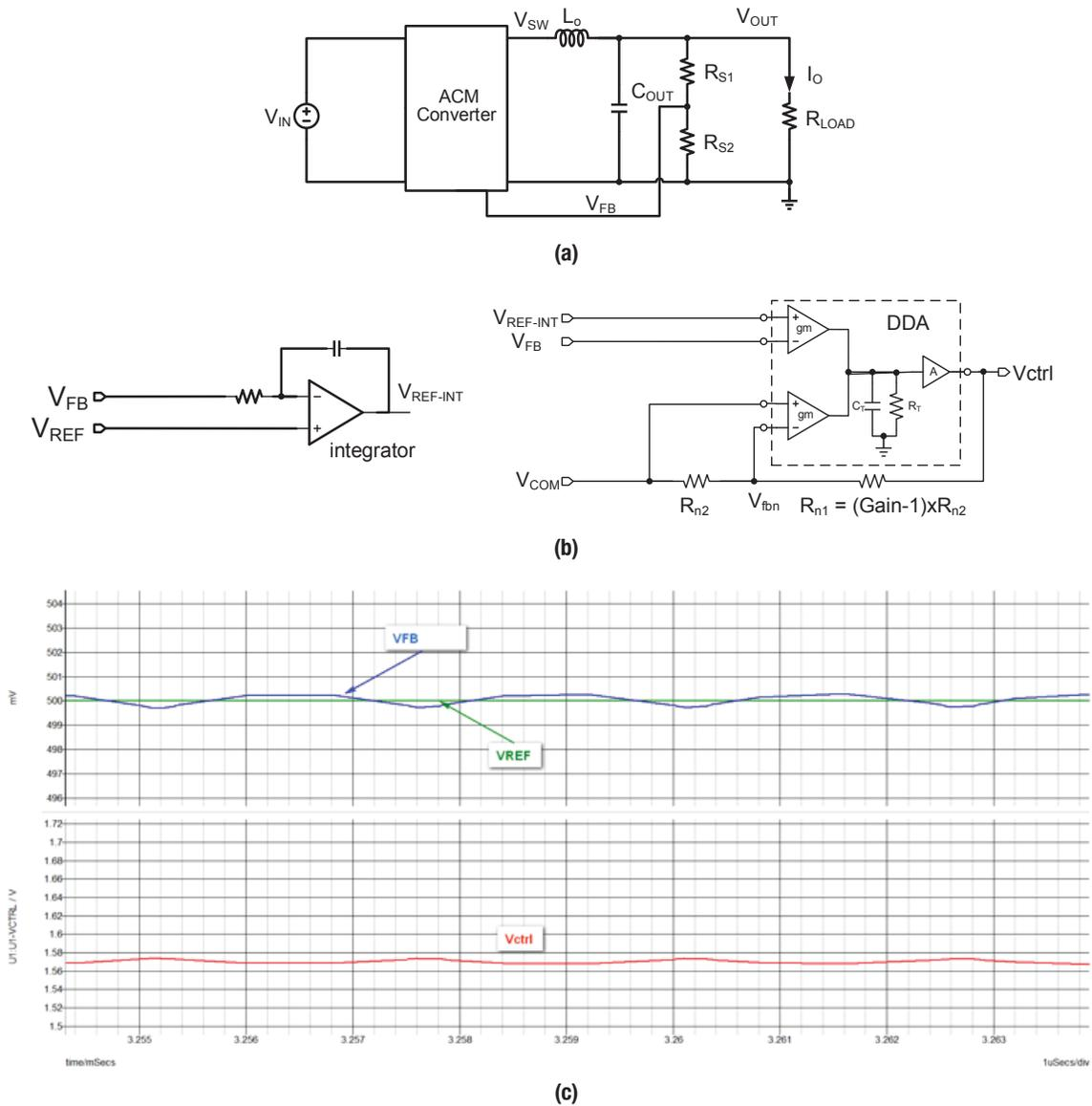
**Figure 4.** Simplified buck converter with ACM (a); circuit block for control voltage (b); simulation waveform from  $V_{FB}$  to control voltage (c).
