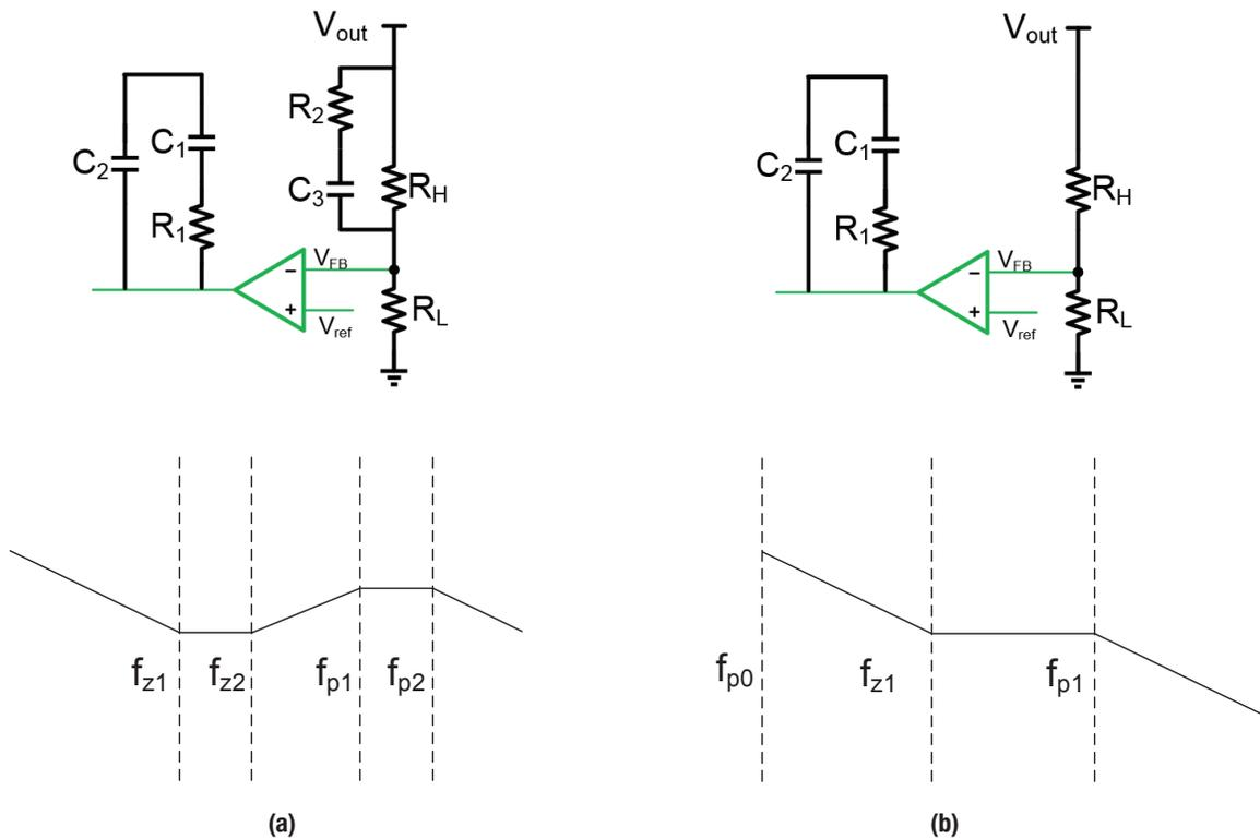
**Figure 2.** Type III compensation for voltage-mode control and compensation curve (a); Type II compensation for current-mode control and compensation curve (b).
