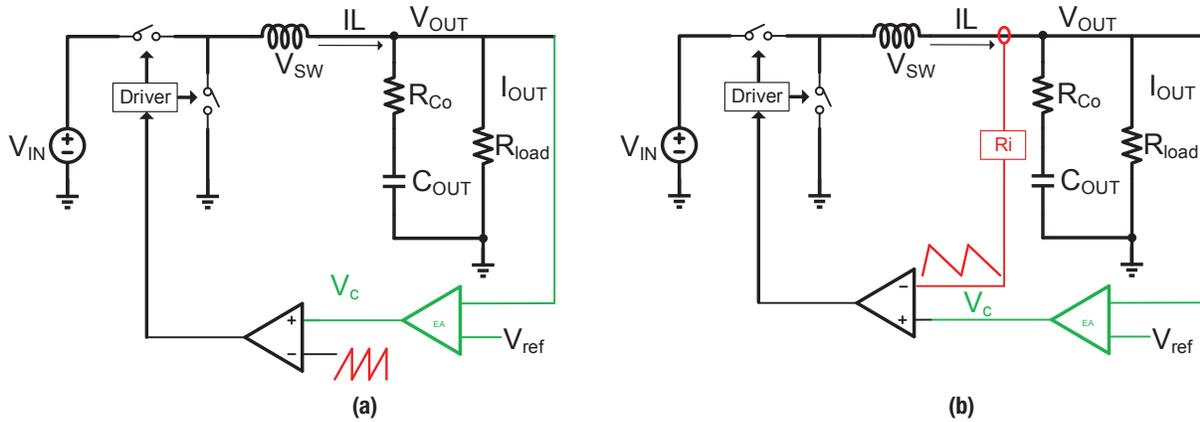
**Figure 1.** Control structure: voltage-mode control (a); current-mode control (b).
