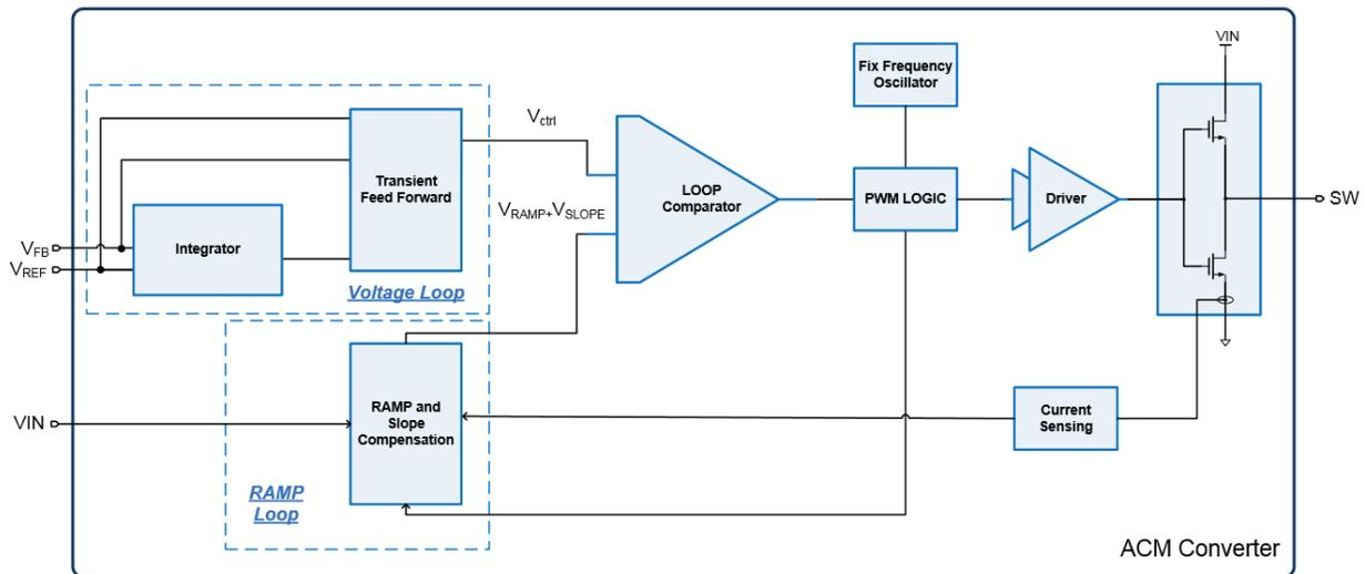
**Figure 5.** ACM control block diagram.
