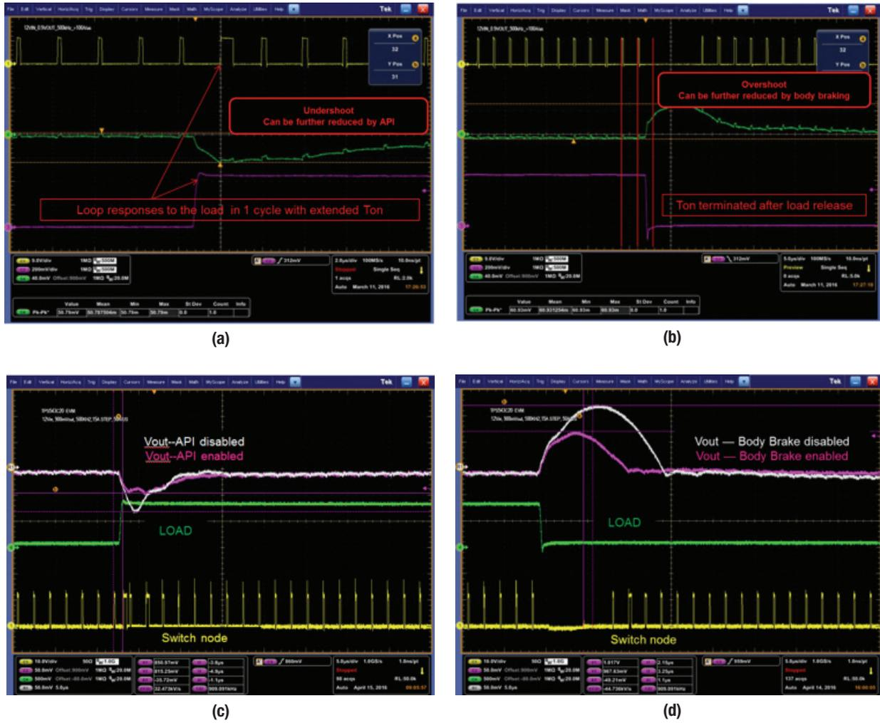
**Figure 8.** Load step-up response (a); load step-down response (b); comparing asynchronous pulse insertion/body brake enable and disable (c) and (d).
