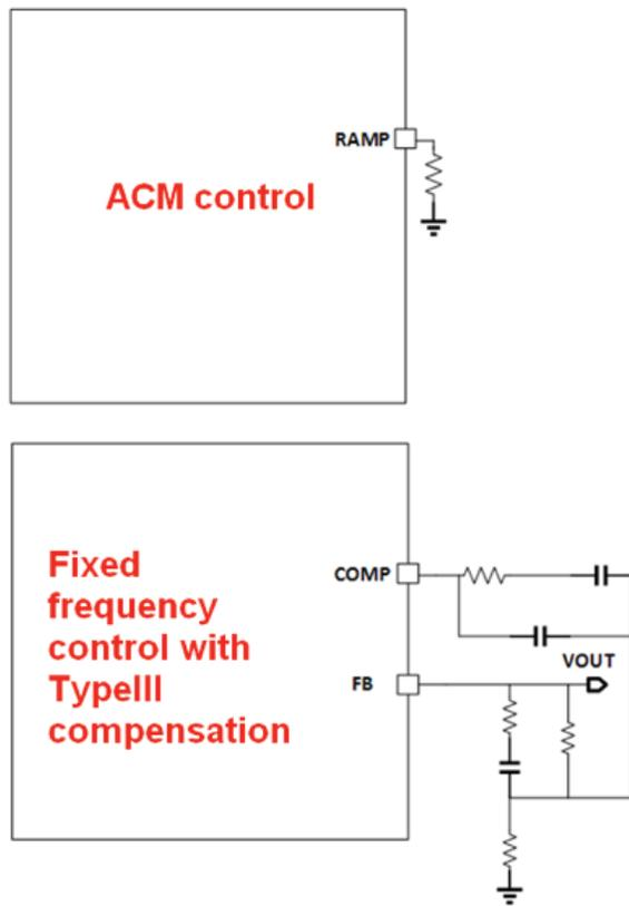
**Figure 9.** Compensation example for ACM control and traditional control, which requires Type III compensation.
