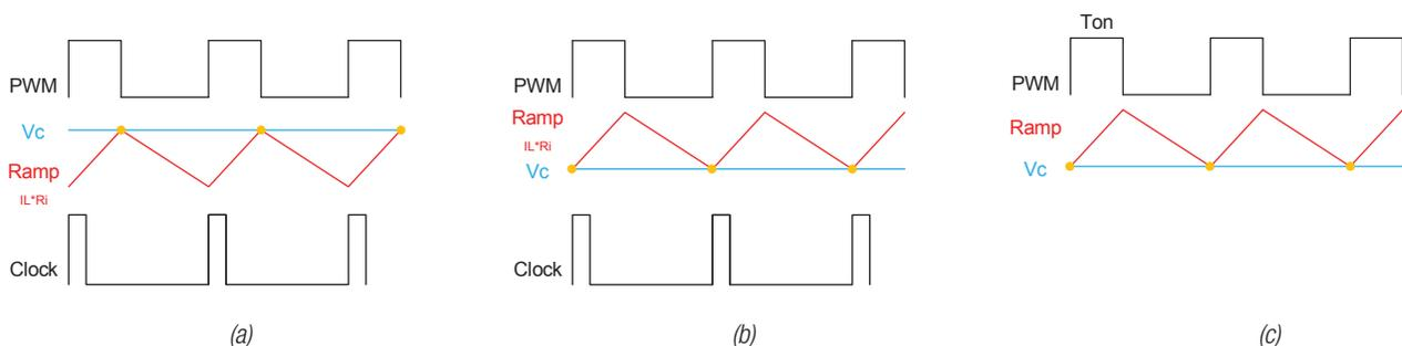
**Figure 3.** Control scheme waveform: PCM (a); valley current mode (b); COT (pseudo current mode) (c).
