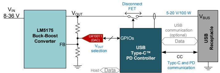
**Figure 5:** USB power provider and data implementation using a four-switch buck-boost and Type-C PD controller.
