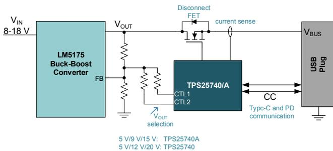
**Figure 4:** An USB PD power provider/charger implementation using a four-switch buck-boost and USB PD controller [8].
