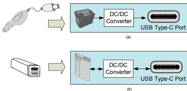
**Figure 1:** USB charging devices include a USB port in a car or a portable USB car charger (a); and a portable rechargeable battery/power bank (b).
