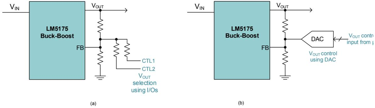
**Figure 3:** Resistor (a) and DAC-based (b) schemes for changing the output voltage of a four-switch buck-boost converter and/or power bank (b).
