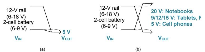
**Figure 2:** Non-PD implementation only requires a step-down conversion (a); PD implementation requires step-up/down conversion in a car charger or power bank (b).
