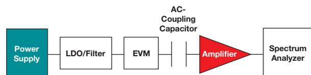
Figure 1. Block diagram of noise measurement setup.
