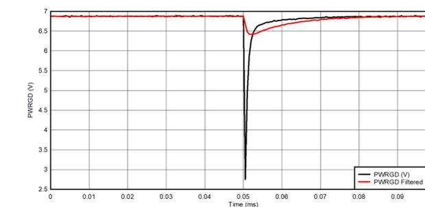
Fig. 10. Typical PWRGD Upset With and Without Filtering.
