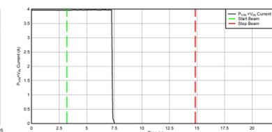
Fig. 7. Typical Current vs Time Plot for a destructive Run of the TPS7H4001-SP at T= 125 C.
