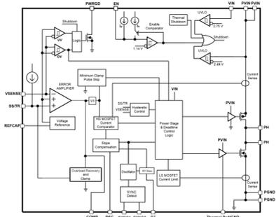
Fig. 2 TPS7H4001-SP functional block diagram.
