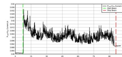
Fig. 6. Typical Current vs Time Plot for a Non-destructive Run of the TPS7H4001-SP at T= 125 C.
