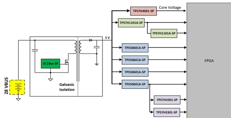
Fig. 1 Typical power distribution for a space rated FPGA, the TPS7H4001-SP for core voltage and TI space grade power solution
