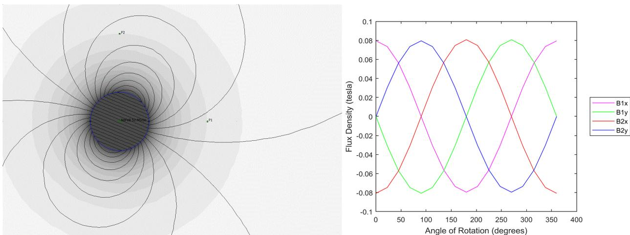
Figure 4. Generating Sinusoidal Magnetic Flux Density Signals
