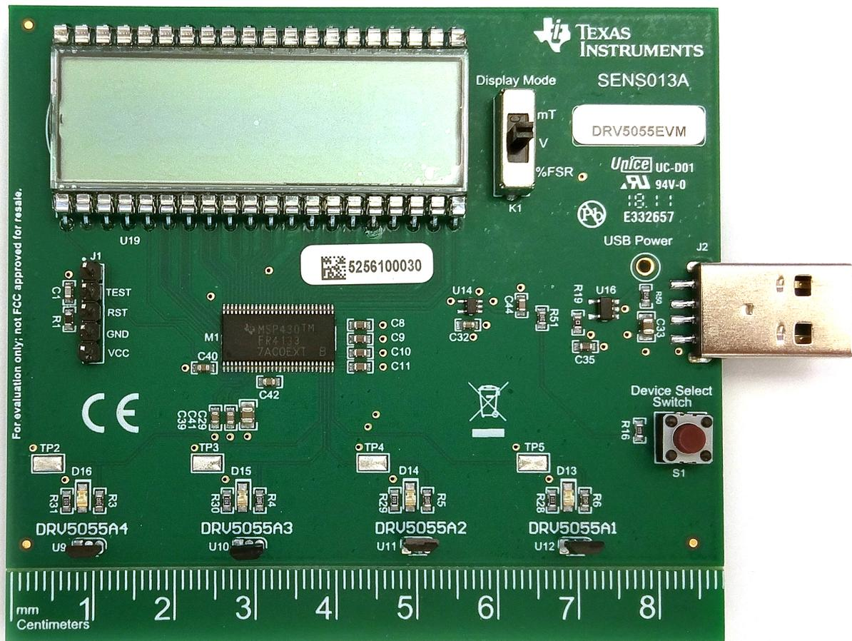
This user's guide describes the characteristics, operation, and use of the [DRV5055](#) evaluation module (EVM). This EVM is designed to evaluate the performance of the DRV5055 ratiometric, linear, Hall effect sensors. Throughout this document, the terms evaluation board, evaluation module, and EVM are synonymous with the DRV5055EVM. This document includes a schematic, reference printed circuit board (PCB) layouts, and a complete bill of materials (BOM).
