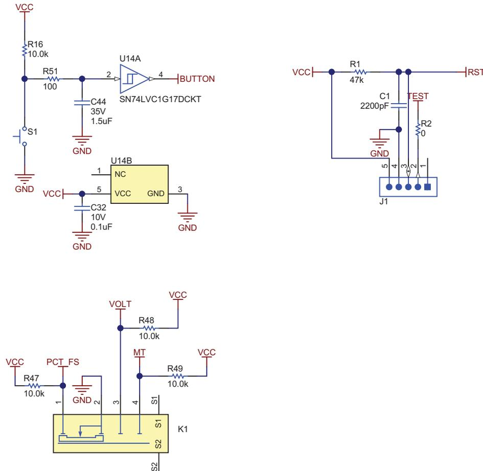
Figure 4. Schematic of Push-Button User Input, Slider Switch User Input, and Programming Input
