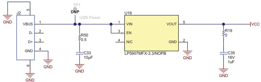
Figure 6. Schematic of Supply Input and Power Conditioning
