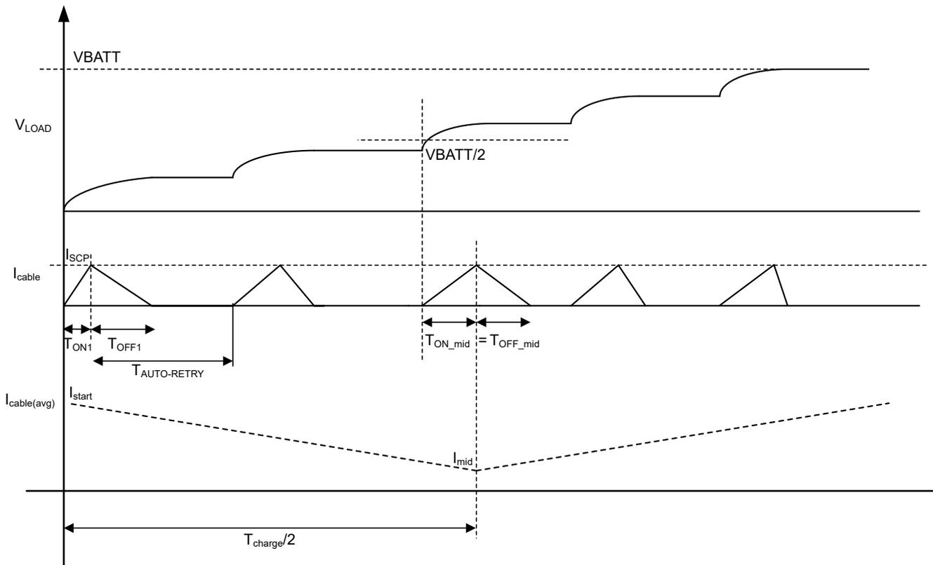
Figure 6. PWM charging method conceptual waveforms during startup.
