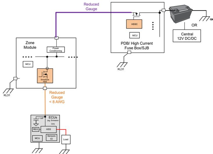
**Figure 2.** Zone-based Power distribution architecture.
