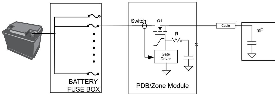
Figure 3. Circuit for output voltage slew-rate control.
