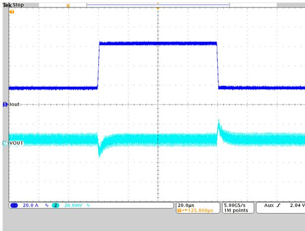
**Figure 3.** The transient response of fixed-frequency DCS-Control is tunable to the most severe load transients, where it provides excellent regulation.
