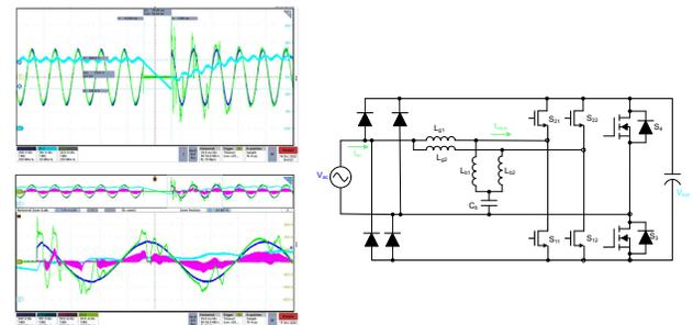
Figure 5. AC dropout and restore performance at 5 kW.
