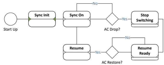
Figure 4. AC dropout and restore state machine.
