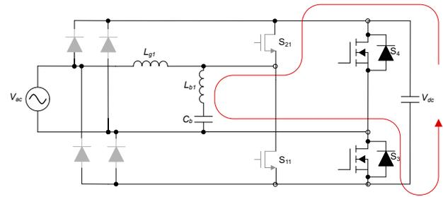
**Figure 2.** Synchronous rectifier  $S_{21}$  delayed turnoff  $V_{dc}$  discharge path.
