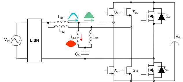
**Figure 1.** iTCM topology with inductor and current envelopes.
