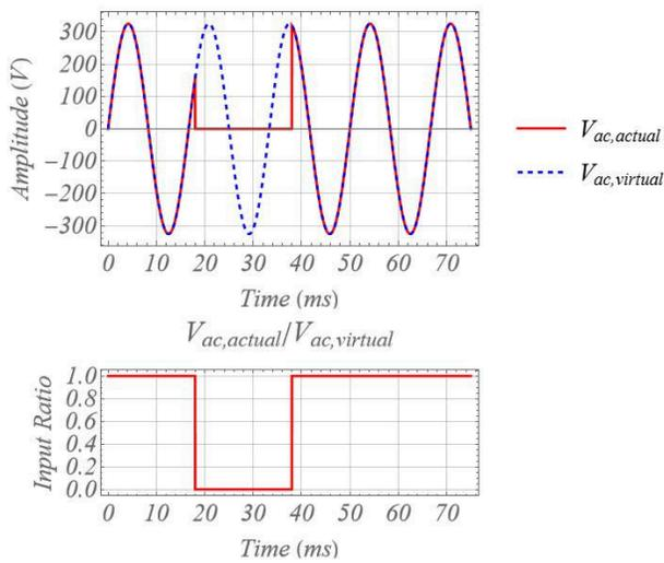
Figure 3. AC input dropout with the virtual AC signal.
