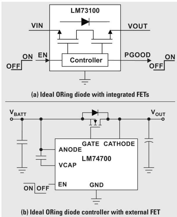
**Figure 4.** Two ORing Configurations
