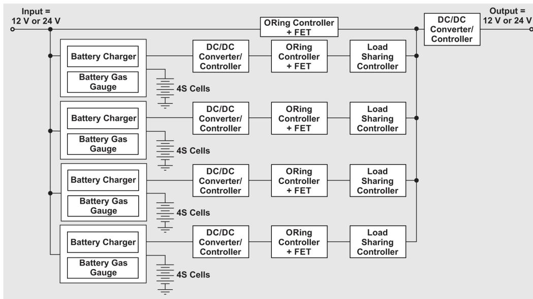
**Figure 2.** Multibattery Management System for a 4S4P Battery Pack
