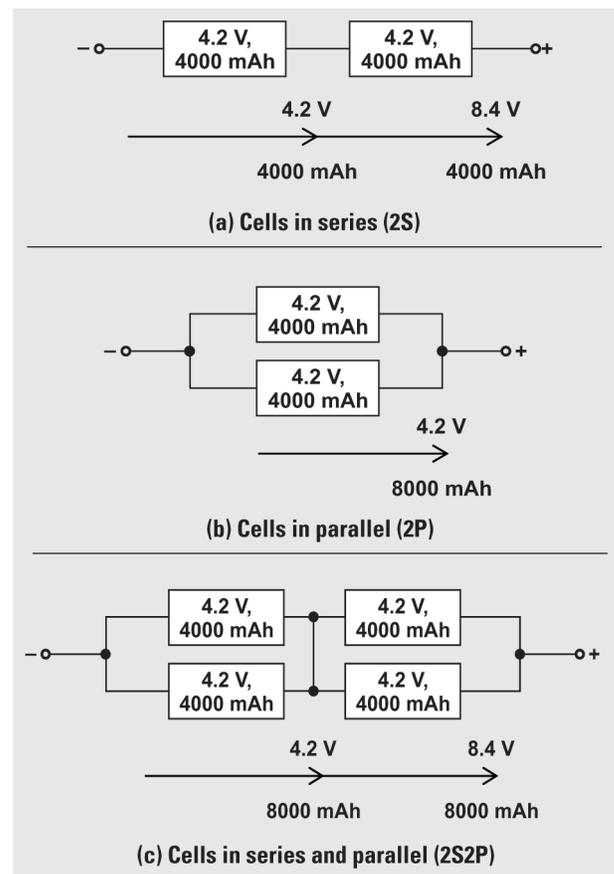
**Figure 1.** Voltage and Capacity Scaling for a Li-ion Battery
