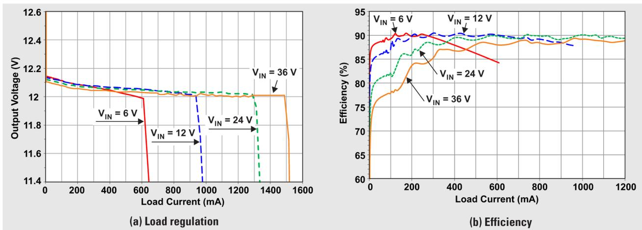
Figure 4. PSR Flyback Converter Performance with a 12-v Output
