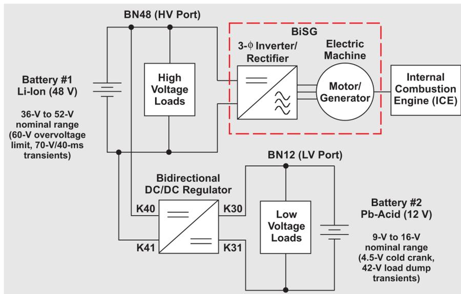
**Figure 1.** Simplified Example of a mHEV Dual-battery System
