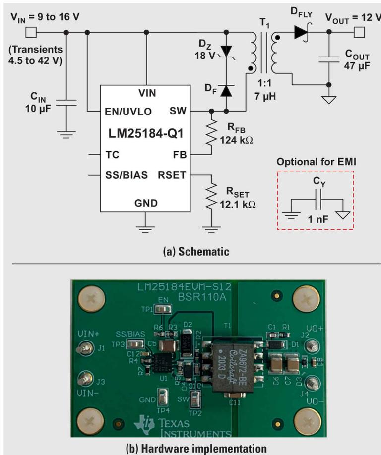
**Figure 3.** Auxless PSR Flyback Converter with a 12-V Output
