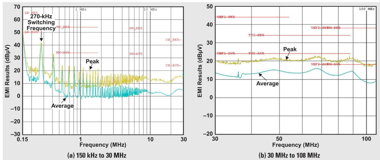
Figure 5. CISPR 25 Class 5 EMI Measurements of the PSR Flyback Converter ( $V_{IN} = 13.5\text{ V}$ ,  $I_{OUT} = 700\text{ Ma}$ )
