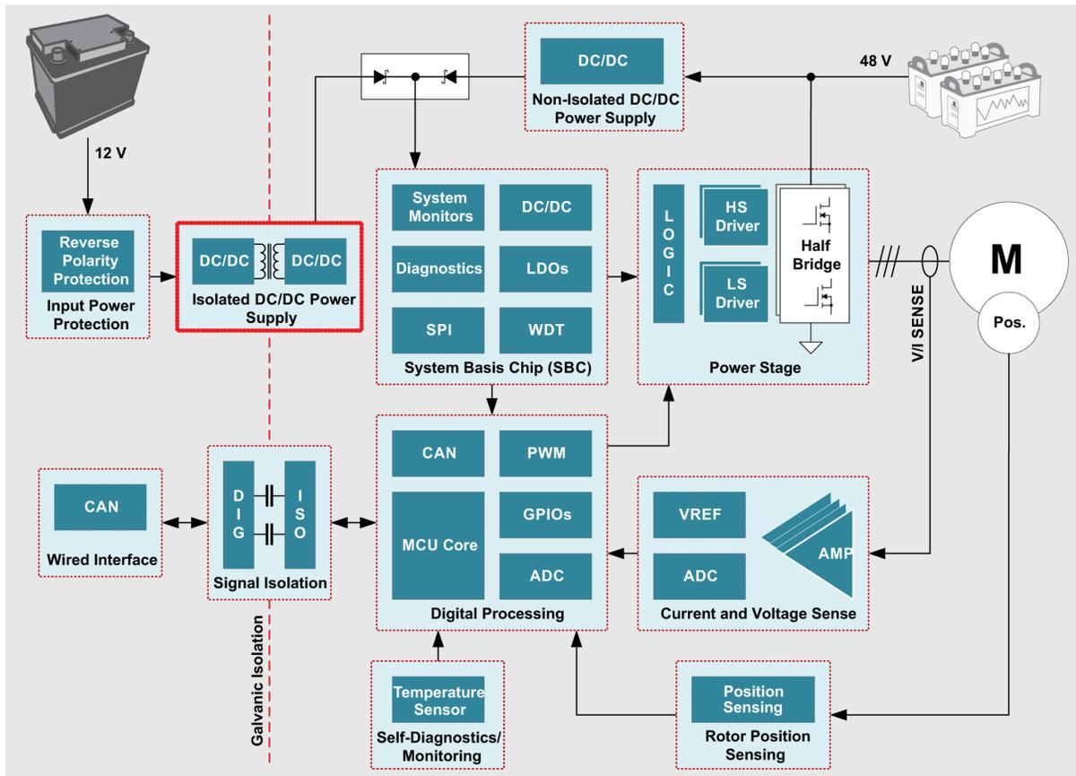
**Figure 2.** Block Diagram of a Starter-generator System (Isolated DC/DC Stage Highlighted in Red)
