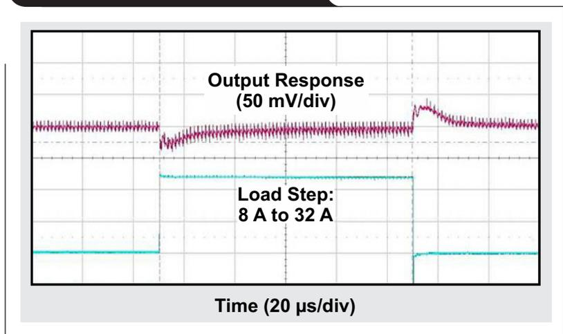
Figure 3. D-CAP3™ transient response
