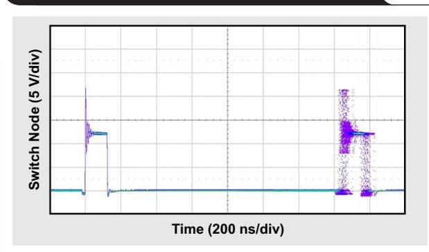
ACM uses a fixed-frequency scheme that improves the frequency jitter performance over the D-CAP3 control mode, as shown in Figure 7. For applications that need more predictable switching-frequency behavior, ACM is the better choice.
