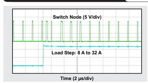
**Figure 5. D-CAP3 switch-node waveform during an 8-A to 32-A load step**
