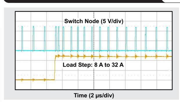
**Figure 6. D-CAP3 frequency jitter at 15 A**
