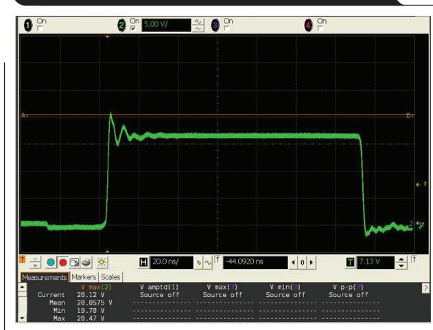
There could be two  $V_{IN}$  spikes during the transient: the first spike is related to the  $ESR_B$ ; and the second spike is caused by the difference between the buck-converter input current ( $\tilde{i}_{IN\_D}$ ) and the bus-converter output current ( $i_{PS}$ ). Both spikes should be lower than the  $V_{IN}$  undershoot or overshoot requirement ( $V_{IN\_tran}$ ).
