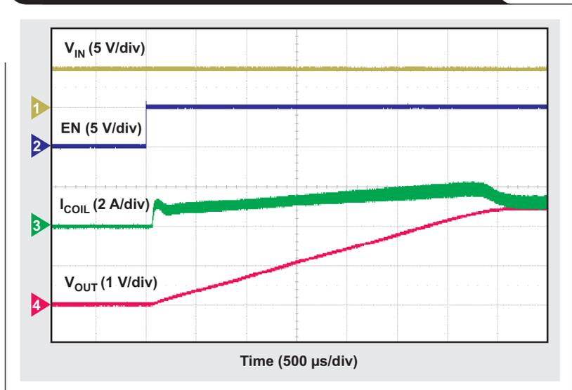
module can start up as usual without the heavy load current or the large amount of output capacitance. Alternatively, the power module can remain always on because the load switch will provide the soft-start function. Figure 5 shows an example implementation with an always on power module and the TPS22954 load switch.
