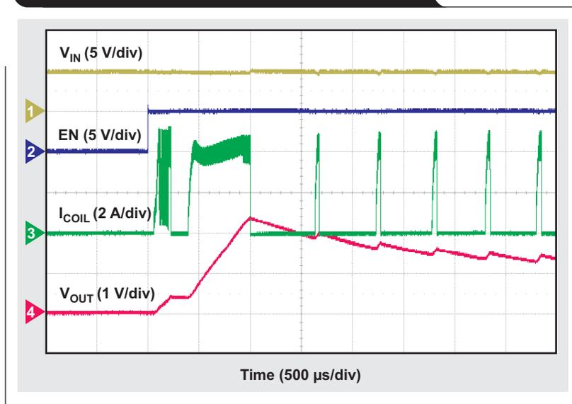
converge to create a system-startup issue. Figure 1 shows the startup of a power module with a 5-V input voltage, the output voltage set to 2.5 V, and two 470-μF capacitors added to the output.<sup>[1]</sup> With a 1-A resistive load added to the output, the output voltage never enters regulation because of current-limit and hiccup current-limit protection. Thus, the device remains in hiccup current-limit operation.
