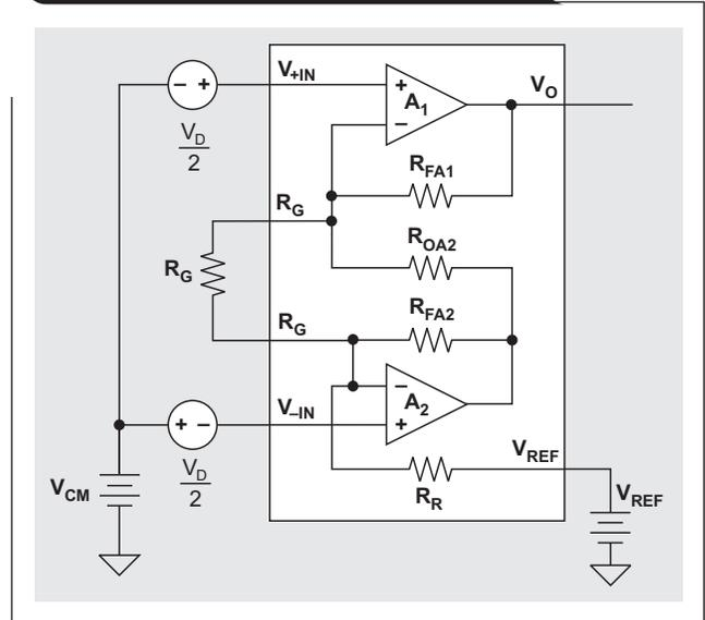
Figure 4. CMRR of two-op-amp vs. three-op-amp topologies
