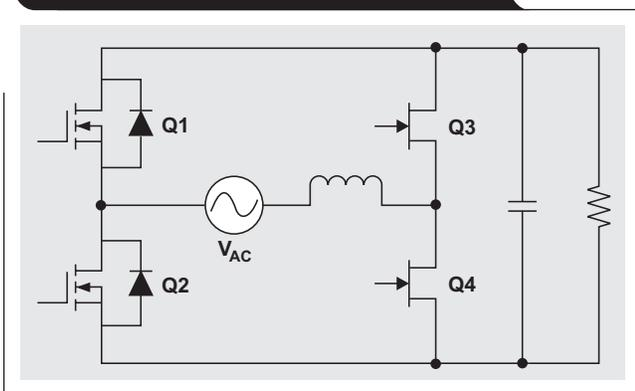
Figure 3. Current paths for positive AC cycle
