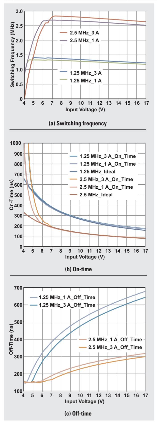
The 2.5-MHz curves in Figure 4b clearly show a minimum on-time in the 80-ns range. This sets an upper boundary on the achievable switching frequency. The 1.25-MHz curves show good frequency variation similar to Figures 2a and 3a. Due to smaller on-times with this 1.8-V output, fixed propagation delays cause a sharper downward frequency shift versus higher output voltages, which result in a lower frequency.
