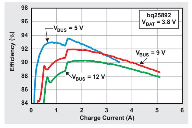
With a 9-V input adapter, a battery charger with 91% efficiency was set to provide a 3-A charging current to a 3.8-V charged battery with losses of
