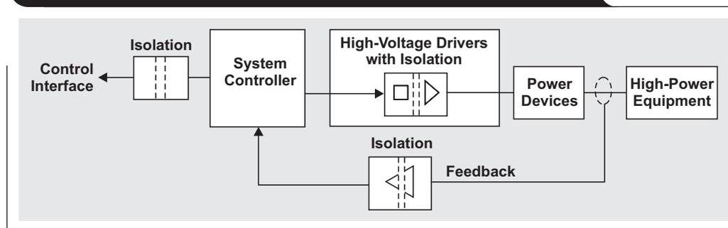
Figure 2. New motor drive architecture
