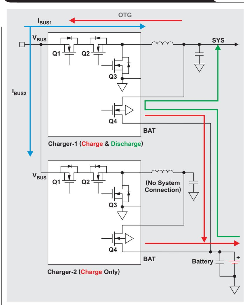
optimization (ICO) to extract maximum adapter power without causing loop instability at their mutual  $V_{BUS}$  node. Therefore, each charger's current-limit feature should be set to half the adapter's maximum output current. Inductor current ratings may also be reduced by half as well.
