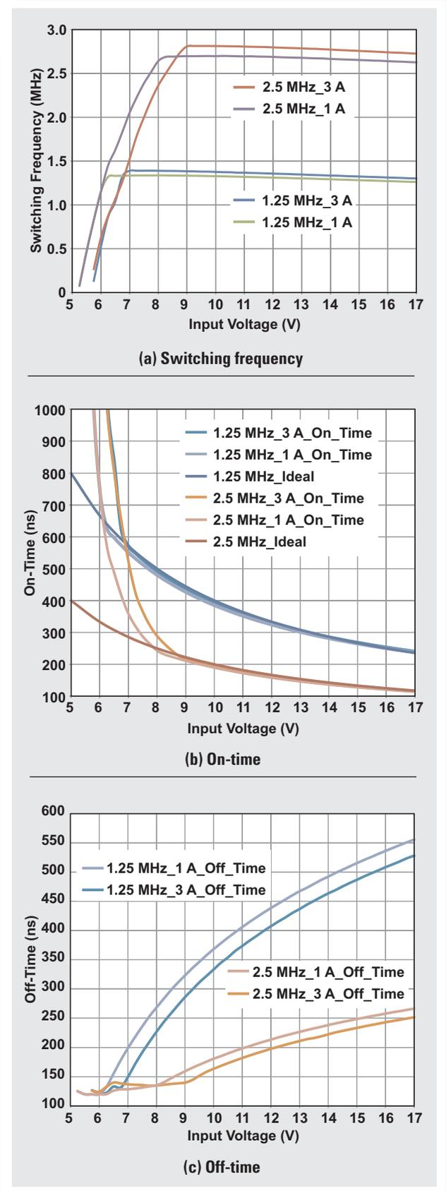
Figure 3 shows measured data for a 3.3-V output. When the input voltage of the converter drops, the duty cycle increases. At high duty cycles, the switching frequency decreases due to losses and a minimum off-time. High duty cycles refers to the left-most portion of Figures 2a and 3a where the switching frequency decreases from its nominal value towards zero.
