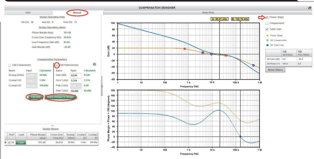
**Figure 6. Bode plot with mixed output capacitors after manual compensation shows increased bandwidth and good phase margin**
