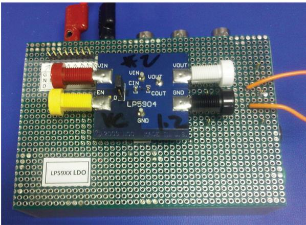
**Figure 3. Back side of LDO test jig**
