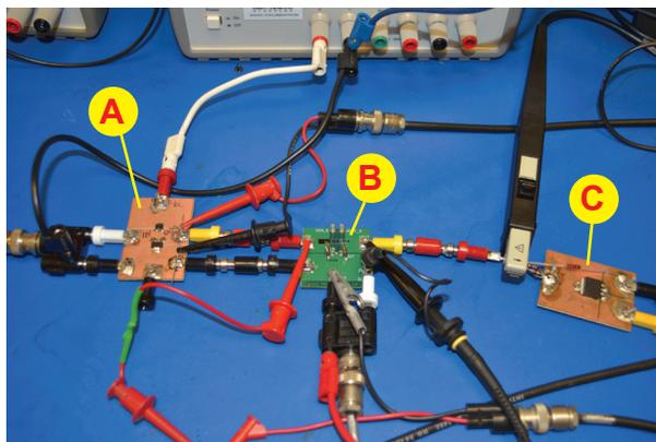
A. Emitter followers and pulse generator create  $V_{IN}$  step voltage during line transient tests.
