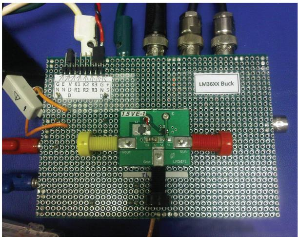
**Figure 6. Back side of buck-regulator test jig**
