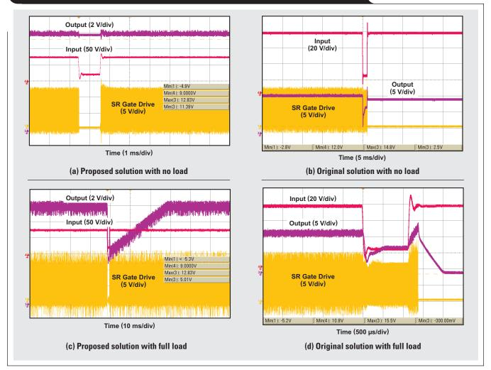
Figure 7. Test results when the input-voltage transient is between 60 V and 20 V  $\,$
