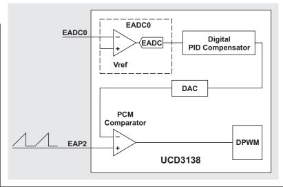
PCM comparator terminates the pulse of the primary gate driver when the sawtooth voltage on the EAP2 pin exceeds the DAC's output. DPWM3A is a complementary signal of the primary gate driver that is generated by the digital controller. This controller is used to discharge C1 at every half switching cycle. R2 is added to limit the voltage on the EAP2 pin, which is lower than its maximum voltage rating at any condition.
