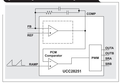
Figure 1. Analog controller with PWM generation
